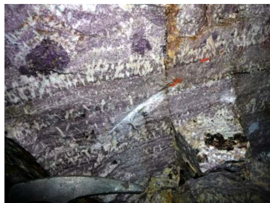
An example of lithium-rich rock called pegmatite, with a characteristic purple colour and which is composed of lithiniferous micas, feldspar and quartz. Chédeville (Haute-Vienne). The pick of a geologist's hammer indicates the scale. E. Gloaguen (BRGM), CC BY-NC-SA
