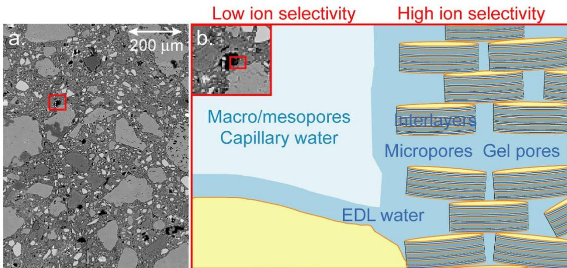
**Fig. 5.** a. Backscattered electron (BSE) image of low-pH cement (modified, from Gaboreau et al. [8]). The brightest parts represent the highest Ca weight %, the anhydrous phases appear in light gray, the hydraulic binder (mostly C-S-H) and silica grains appear in dark gray, and the macropores appear in black. b. Close-up of the pore structure of low-pH cement showing the zones with low and high ion selectivity (modified, from Jennings [101]).
