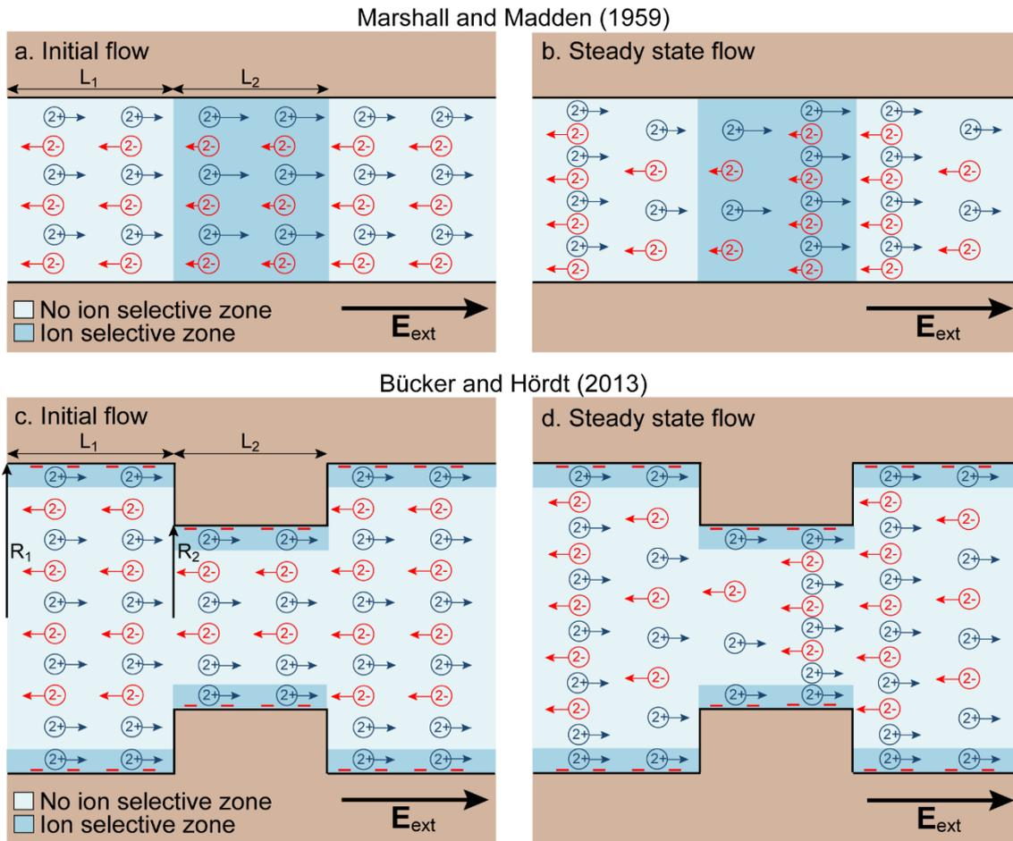
**Fig. 6.** Sketch of the membrane polarization model of Marshall and Madden [76] (a, b) and Bücker and Hördt [42] (c, d) when the porous medium containing a  $\text{CaSO}_4$  aqueous electrolyte is under the influence of the external electric field  $\mathbf{E}_{\text{ext}}$ . In steady state conditions, ion concentration gradients due to the ion selectivity in the membrane zone appear. The length of the arrow depicted for the ions denotes the magnitude of the ion mobility.
