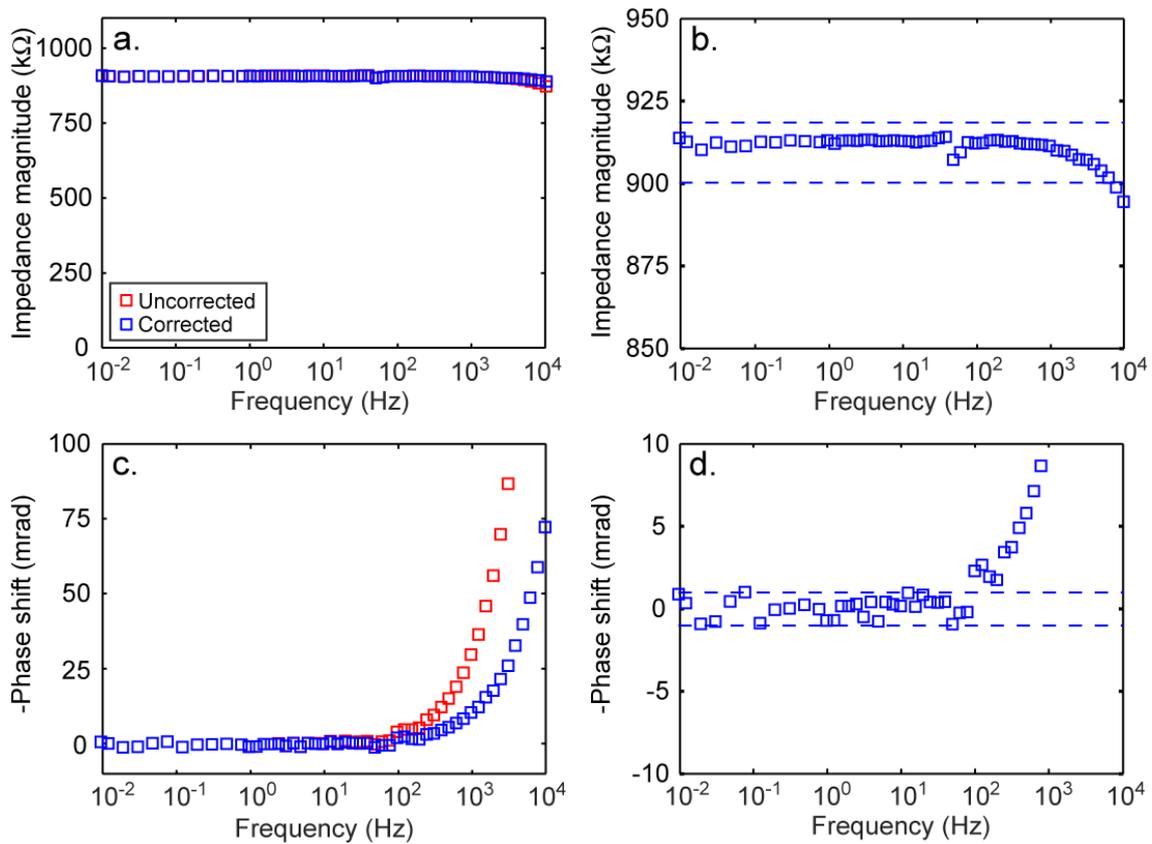
**Fig. 3.** Complex impedance measurements on a reference electrical circuit. Ideally, the magnitude of the measured impedance should be 909  $k\Omega$  with zero phase shift.
