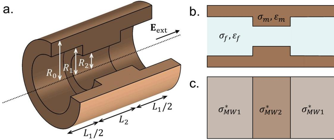
**Fig. 7.** a. Cylindrical model consisting of the wide pore (length  $L_1$ , radius  $R_1$ ), narrow pore (length  $L_2$ , radius  $R_2$ ) and non-conducting matrix (thickness  $R_0 - R_1$  or  $R_0 - R_2$ ). b. Cross-section through the pore system showing the pore and surrounding matrix conductivity and permittivity. c. Reduction of b. to a layered medium with effective complex Maxwell-Wagner conductivities (after Bucker [84]).
