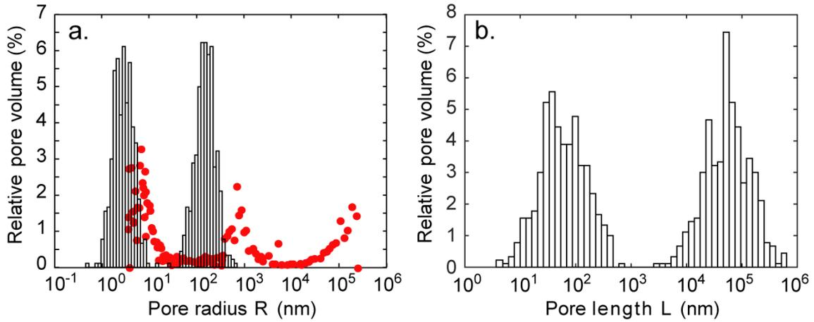
**Fig. 12.** a. Pore radius distribution and b. pore length distribution used in the network model to match the SIP measurements on HCP. Filled red circles are the pore radii measurements from MIP (Fig. 1). The distributions used in the network model to match the SIP measurements on concrete look similar and are not shown for brevity.
