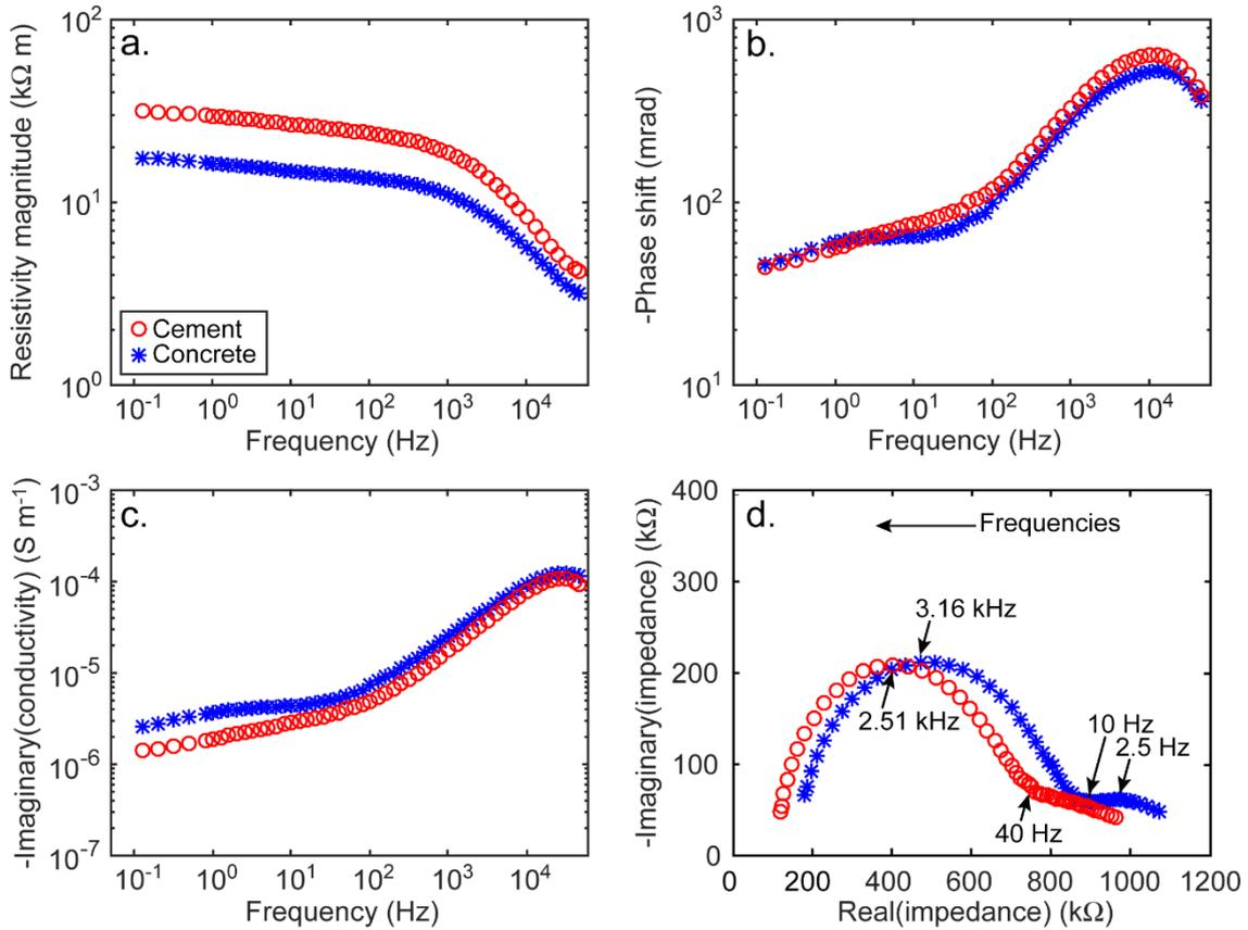
**Fig. 9.** Measured HCP and concrete SIP spectra (symbols).
