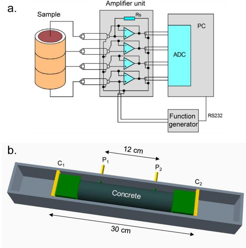
**Fig. 2.** a. Sketch of the ZEL-SIP-04 system (modified, from Zimmermann et al. [38]). b. Sketch of the sample holder for SIP measurements on concrete. Synthetic wet sponges (light green) were used to establish contact between the current ( $C_1$ ,  $C_2$ ) and potential ( $P_1$ ,  $P_2$ ) electrodes and the sample (dark green).
