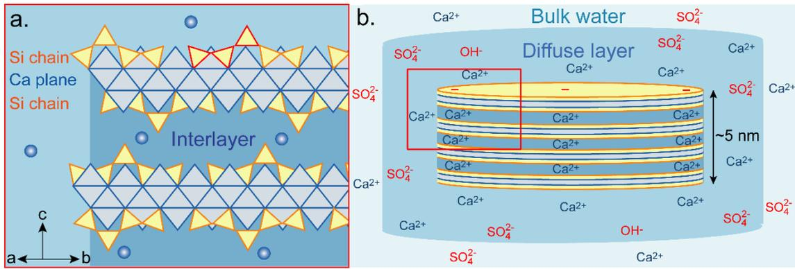
**Fig. 4.** a. Close-up of a C-S-H particle in a calcium sulfate aqueous electrolyte. The dreierketten structure of the silicate chains is drawn in red (modified, from Grangeon et al. [108]). b. Diffuse layer around the C-S-H particle containing calcium cations in excess and sulfate anions in deficiency to compensate the external negative surface charge of C-S-H (modified, from Haas and Nonat [105]).
