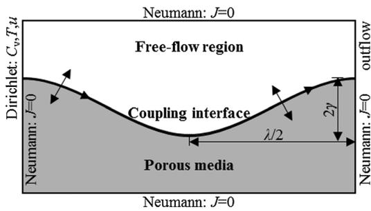
**Figure 1.** Two-dimensional configuration (subdomains and boundary conditions) where  $C_v$  is the water vapor concentration;  $T$  is temperature;  $u$  is wind speed;  $J$  is flux for  $T$ ,  $u$ , and  $C_v$ ;  $\lambda$  is wave length; and  $\gamma$  is half of the wave amplitude.
