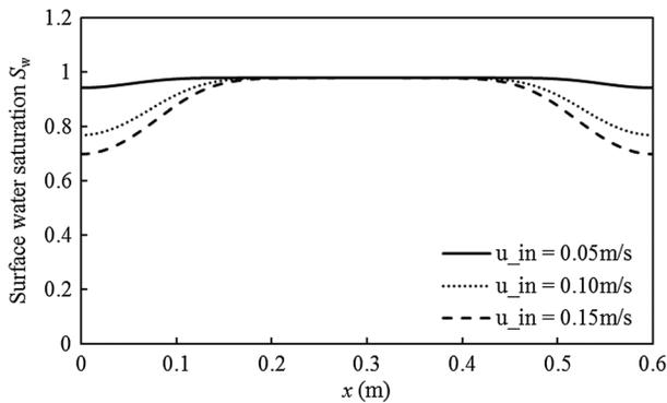
**Figure 10.** Water saturation distribution at the surface during stage I ( $t = 1$  day) under different air flow velocities ( $C_{v,inlet} = 0.006 \text{ kg/m}^3$ ,  $T_{inlet} = 293.15 \text{ K}$ ,  $K = 1\text{E}-10 \text{ m}^2$ ,  $\phi = 0.312$ ,  $\alpha = 8$ ,  $n = 5$ ,  $AR = 1/6$ ).
