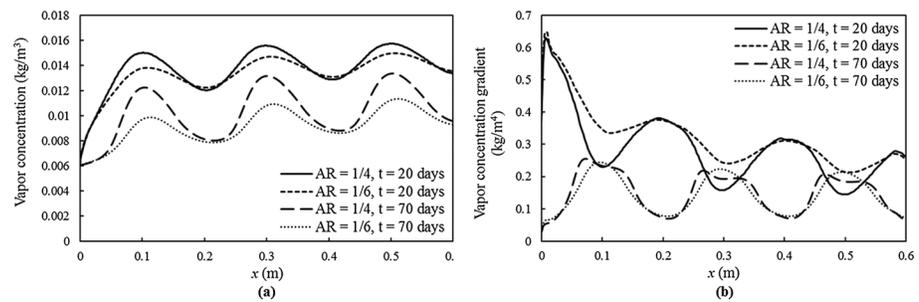
**Figure 14.** (a) Vapor concentration along soil surface with AR of 1/6 and 1/4 at  $t = 20$  and 70 days. (b) Normal vapor concentration gradient along soil surface with AR of 1/6 and 1/4 at  $t = 20$  and 70 days. AR = aspect ratio.
