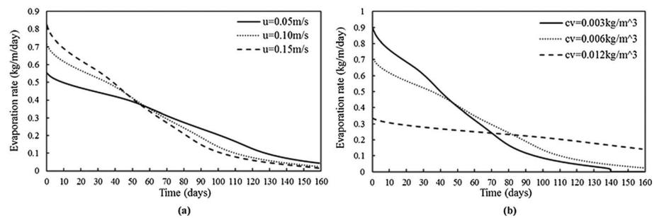
**Figure 9.** (a) Impact of air flow velocity (wind speed) on evaporation rate ( $C_{v,inlet} = 0.006 \text{ kg/m}^3$ ,  $T_{inlet} = 293.15 \text{ K}$ ,  $K = 1\text{E}-10 \text{ m}^2$ ,  $\phi = 0.312$ ,  $\alpha = 8$ ,  $n = 5$ ,  $AR = 1/6$ ). (b) Effect of ambient vapor concentration on evaporation rate ( $u_{inlet} = 0.10 \text{ m/s}$ ,  $T_{inlet} = 293.15 \text{ K}$ ,  $K = 1\text{E}-10 \text{ m}^2$ ,  $\phi = 0.312$ ,  $\alpha = 8$ ,  $n = 5$ ,  $AR = 1/6$ ).
