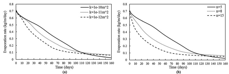
**Figure 11.** (a) Effect of intrinsic permeability on evaporation rate ( $u_{g,inlet} = 0.10 \text{ m/s}$ ,  $C_{v,inlet} = 0.006 \text{ kg/m}^3$ ,  $T_{inlet} = 293.15 \text{ K}$ ,  $\phi = 0.312$ ,  $\alpha = 8$ ,  $n = 5$ ,  $AR = 1/6$ ). (b) Effect of van Genuchten parameter  $n$  on evaporation rate ( $u_{g,inlet} = 0.10 \text{ m/s}$ ,  $C_{v,inlet} = 0.006 \text{ kg/m}^3$ ,  $T_{inlet} = 293.15 \text{ K}$ ,  $K = 1\text{E}-10 \text{ m}^2$ ,  $\phi = 0.312$ ,  $\alpha = 8$ ,  $AR = 1/6$ ).
