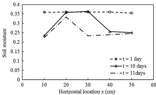
**Figure 7.** The experimental moisture distribution along one horizontal line where the sensors #2, #6, #10, #14, and #19 are located at  $t = 1, 10,$  and  $11$  days. The horizontal location of these five sensors are  $x = 10, 20, 30, 40,$  and  $50$  cm, respectively. Sensors #2 and #19 are  $10$  cm below the wavy surface; sensors #6 and #14 are  $5$  cm below the wavy surface; and sensor #10 is  $2.5$  cm below the wavy surface.
