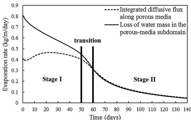
**Figure 8.** Typical evaporation rate curve by coupling model.
