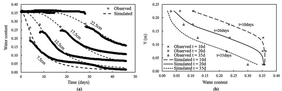
**Figure 4.** (a) Comparison of subsurface moisture evolution with time (rhombus marks in a = the observed data from experiment; dash line = simulated results by modeling) and (b) moisture profile at  $x = 10$  cm.
