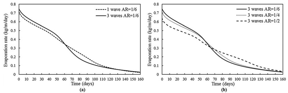
**Figure 12.** (a) Effect of wave numbers on evaporation rate ( $u_{g,inlet} = 0.10$  m/s,  $C_{v,inlet} = 0.006$  kg/m<sup>3</sup>,  $T_{inlet} = 293.15$  K,  $K = 1E-10$  m<sup>2</sup>,  $\phi = 0.312$ ,  $\alpha = 8$ ,  $n = 5$ ). (b) Effect of aspect ratio (AR) on evaporation rate ( $u_{g,inlet} = 0.10$  m/s,  $C_{v,inlet} = 0.006$  kg/m<sup>3</sup>,  $T_{inlet} = 293.15$  K,  $K = 1E-10$  m<sup>2</sup>,  $\phi = 0.312$ ,  $\alpha = 8$ ,  $n = 5$ , 3 waves).
