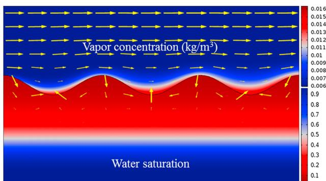
**Figure 13.** Distribution of vapor concentration (kg/m<sup>3</sup>) in the free-flow region and saturation in the porous media (AR = 1/4, the arrows show the gas flows direction and the size of the arrows is proportional to the gas velocity. Separate scales of the arrows are used in free-flow region and porous media).
