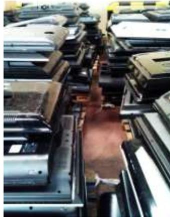
A photo is showing the collected stacks of LCD's on pallets ready for transport. The required collection procedure provides the advantage for separation options to sort the plastic mix after shredding. A similar situation is found for Polystyrene from selectively collected refrigerators.
