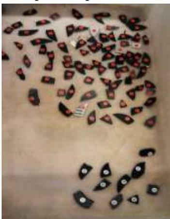
Figure 3 Labeled black plastic particles (5-25 mm size)
