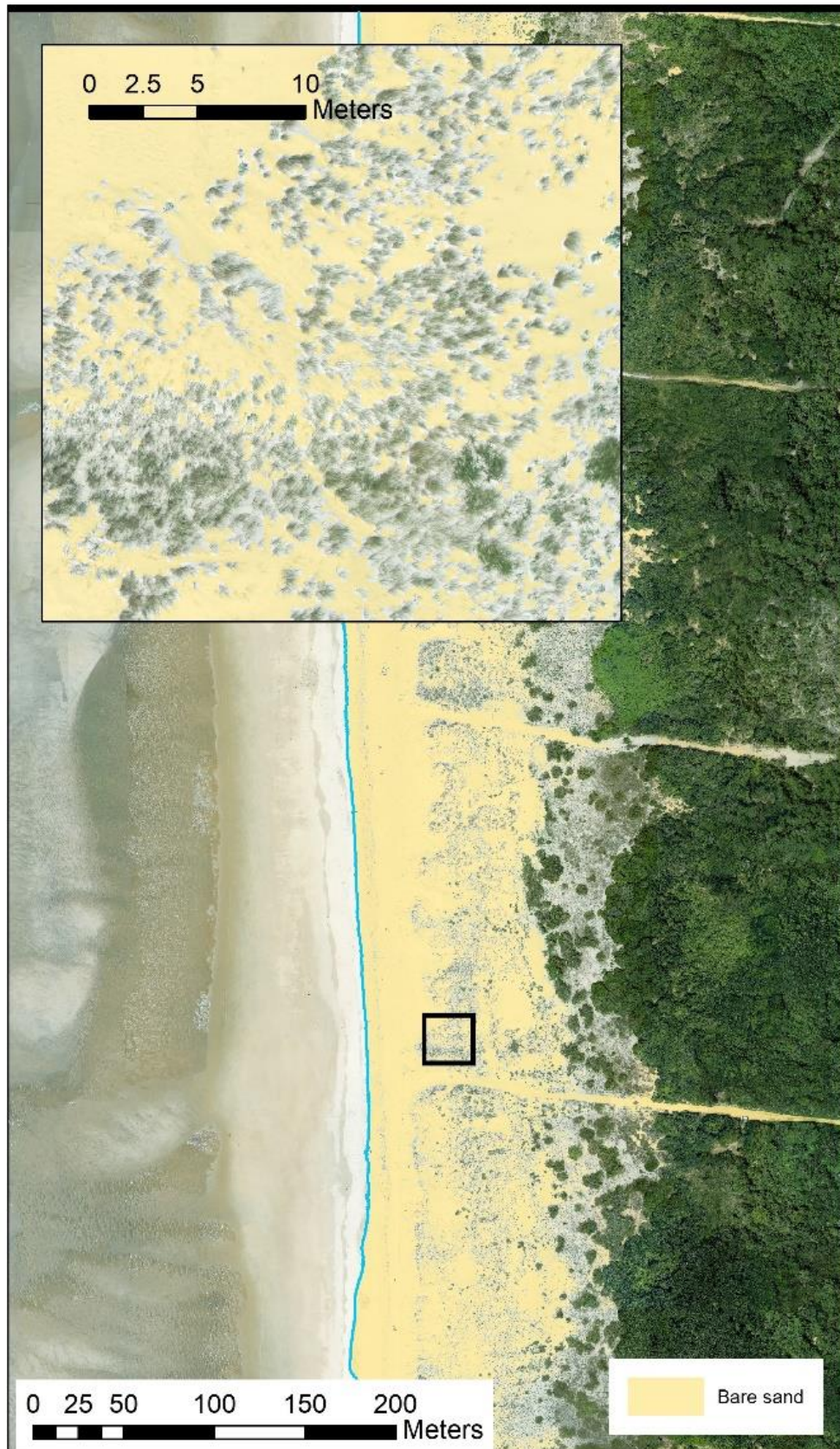
Figure 2. Map of bare sand (yellow) generated by processing of orthophoto at 2 cm of resolution indicating areas prone to aeolian processes
