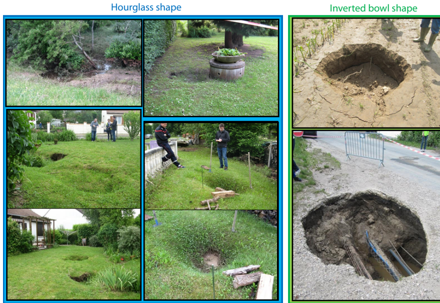
Figure 3: "Post-mortem" shapes of flood-induced sinkholes in Chécý area.
