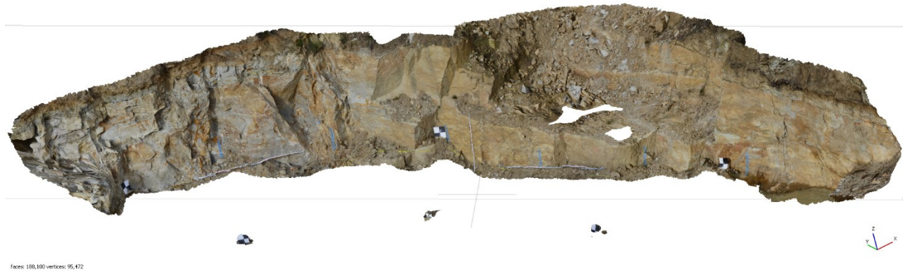
Figure 5: Virtual outcrop model of the targeted rock wall at the Lyas quarry, produced under Agisoft Metashape Professional software. The white zones corresponds to area with not enough images to reconstruct the model. The rods are 5 m long.
