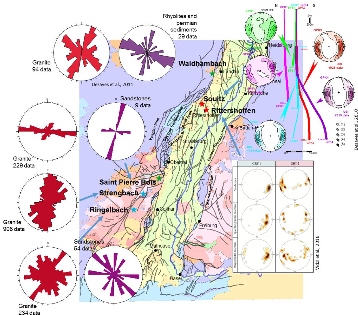
**Figure 3: Orientation of fractures for the different sites. Data for Soultz from Dezayes *et al.*, 2010, Waldhambach from Dezayes *et al.*, 2011 and Rittershoffen from Vidal *et al.*, 2016.**
