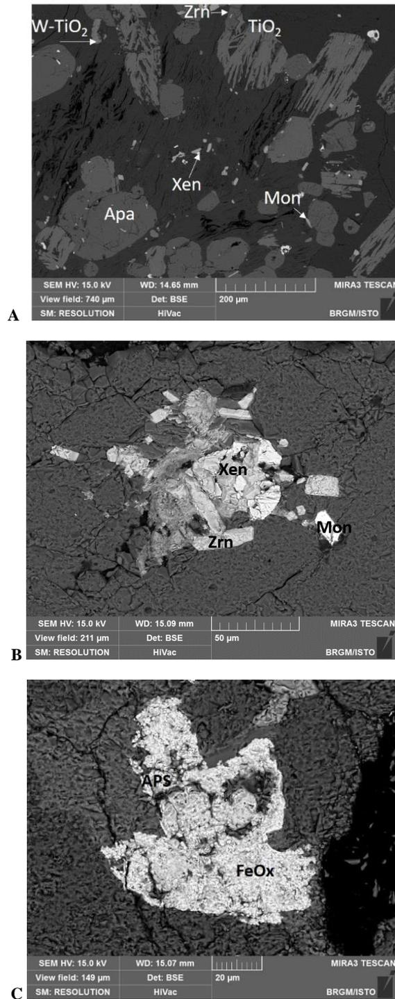
**Figure 4: Backscattered Scanned Electron microscope image of accessory minerals. A- Strengbach; B- Saint Pierre Bois; C- Ringelbach. Zrn zircon, TiO<sub>2</sub> with and without W, Xen xenotime, Mon monazite, Apa apatite, APS aluminum-phosphate-sulfates.**
