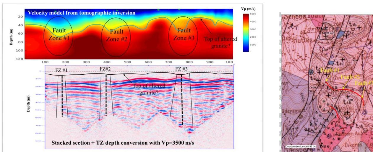
**Figure 8: Results of the 2D reflection seismic profile. Right: geological map of the Ringelbach area with the location of 2D seismic line. Left top: Velocity model derived from the travel-time inversion of first breaks. Bottom: stacked migrated section in depth (Darnet *et al.*, 2019).**
