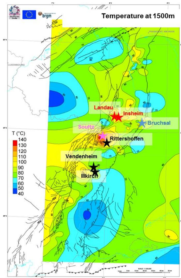
**Figure 1: Present-day and future exploitation geothermal site on temperature map at 1 500 m depth within the Rhine Graben (data from LIAG). The colors of stars indicate the targeted reservoir: red: sedimentary cover-basement transition, pink: granitic basement, black: fault zones at the transition cover-basement zone, blue: deep sediments.**
