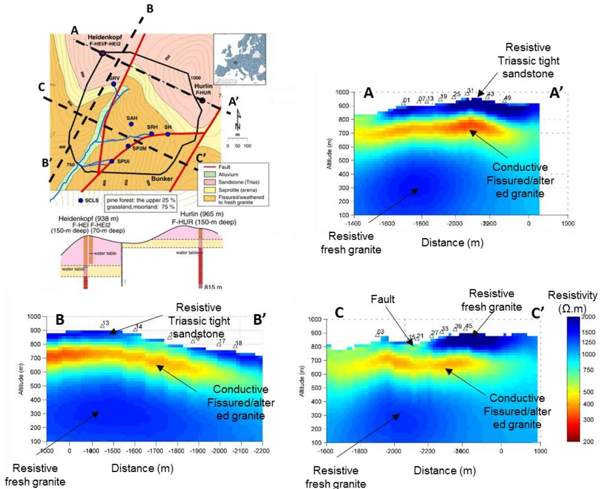
**Figure 7: Results of CSEM inversion Top left: geological map of the Ringelbach area with location of the resistivity cross-sections. Top right and bottom: Resistivity cross-sections A-A', B-B' and C-C' obtained from the inversion of 3D Controlled-Source Electro-Magnetic data (Darnet *et al.*, 2019).**
