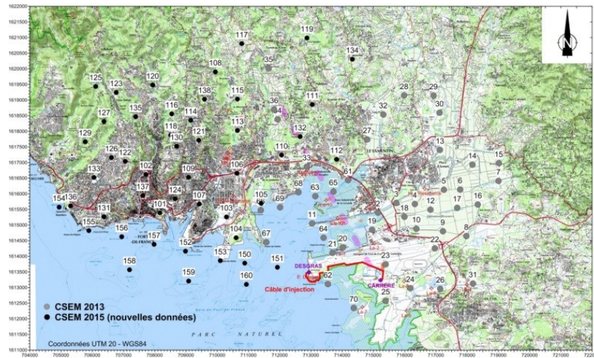
Figure 1: Location of the CSEM recording stations (black dots) and CSEM transmitter (thick red line) acquired of the prospective area of the Lamentin Bay area, next to the Fort de France city. The geothermal field is likely to sit underneath the bay area where several exploratory wells have been drilled (red circles).
