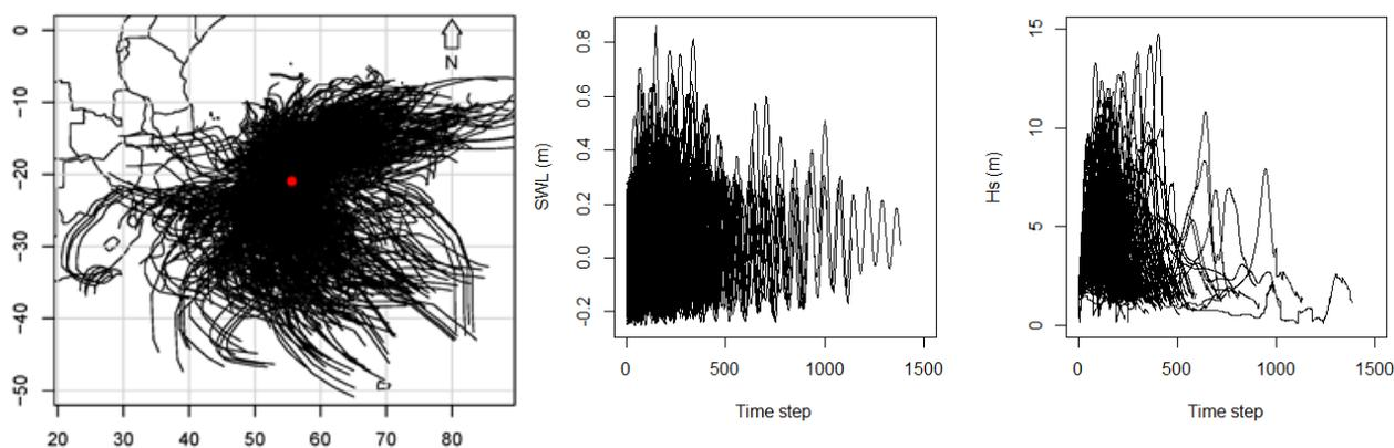
**Figure 3:** 500 synthetic tracks constituting the database with examples of 30 time series (presented on a normalized time index) of significant wave heights (Hs) and seawater levels (SWL) at 50m depth in front of Sainte-Suzanne city.
