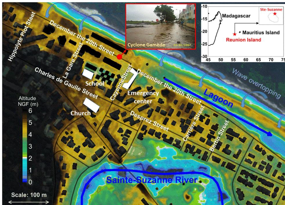
**Figure 1:** Topography of Sainte-Suzanne city derived from high-resolution LIDAR (IGN) data with main streets and critical buildings of the sea-front quarter.
