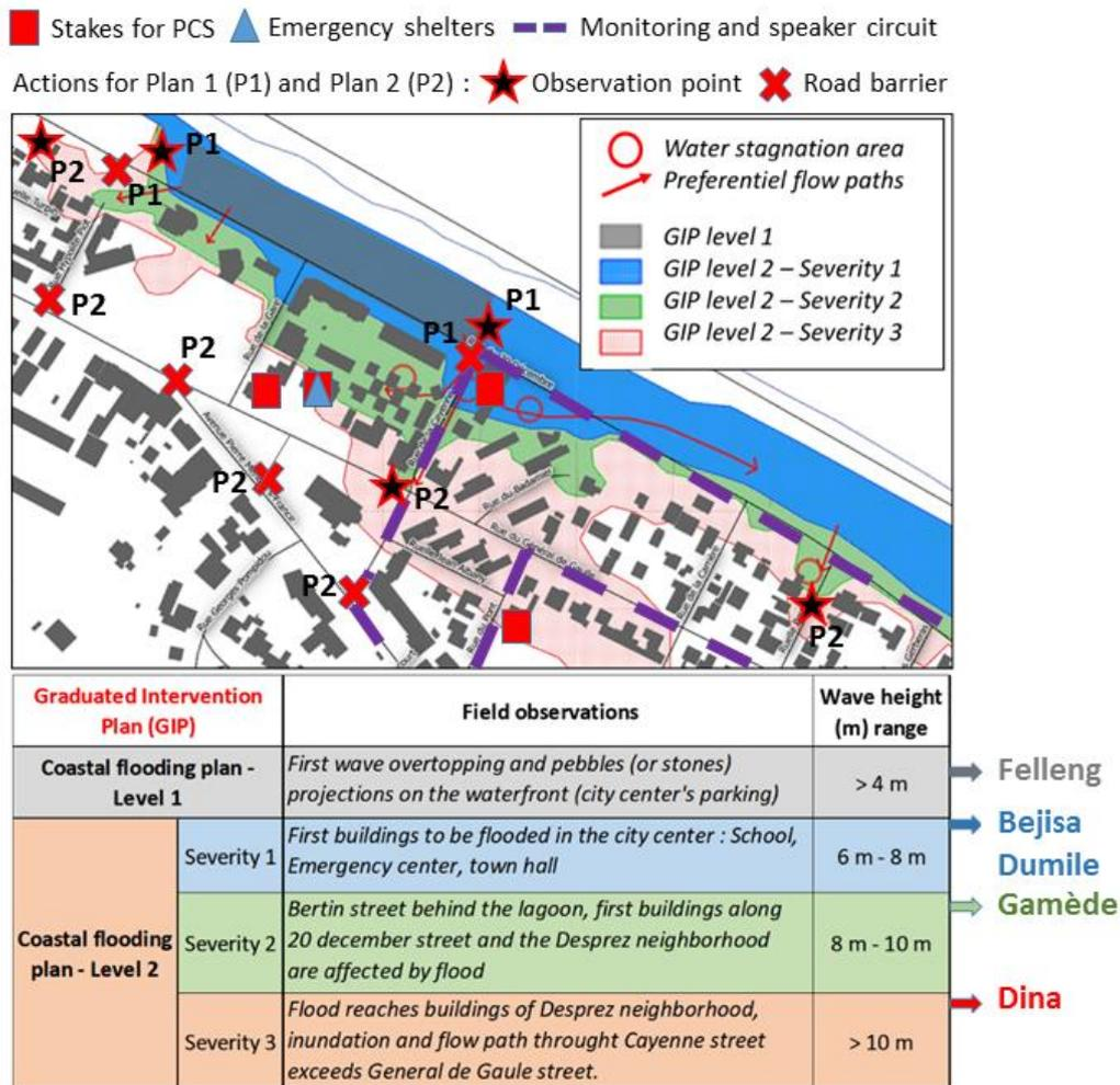
**Figure 6:** Map aggregating the different levels of the Graduated Intervention Plan (GIP) of Sainte Suzanne city centre with the transition criteria (field observations, Hs thresholds and benchmarks).
