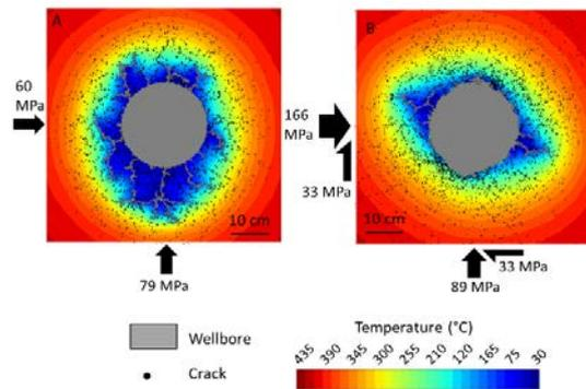
**Figure 3: Thermal fracturing modelled after 4 hours of thermal loading. The front colour corresponds to the temperature (see legend). Each dot corresponds to a crack between two grain-modelling particles. Grey uniform colour corresponds to the area connected to the wellbore (penetration of thermal loading). A: Result for a regional normal faulting regime; B: Result for a strike-slip regime (modified from Peter-Borie et al., 2018).**
