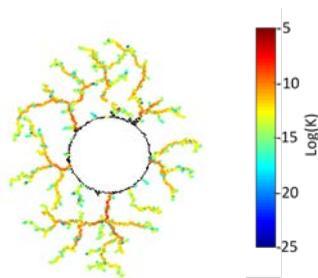
**Figure 4: Logarithm of the permeability ( $K$  [ $m^2$ ]) of the coalesced-cracks discontinuities resulting from the numerical modelling of the thermal loading of the dolerite in the surrounding of the RN-15/IDDP-2 wellbore (see Figure 3A; modified from Tran et al., 2018)**
