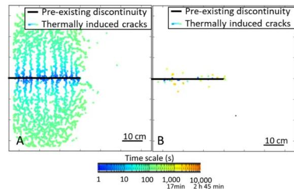
**Figure 8: Thermal failure in a quartz vein (A) and in the plutonic formation (B) at 4775 m depth from the tip of a discontinuity perpendicular to the minimum horizontal stress. The temperature difference between the rock mass and the fluid in the fracture is  $150^\circ\text{C}$ . The colour scale refers to the simulated time from the cold fluid injection in the discontinuity (M. Peter-Borie, unpublished results from Soultz-sous-Forêts investigations).**
