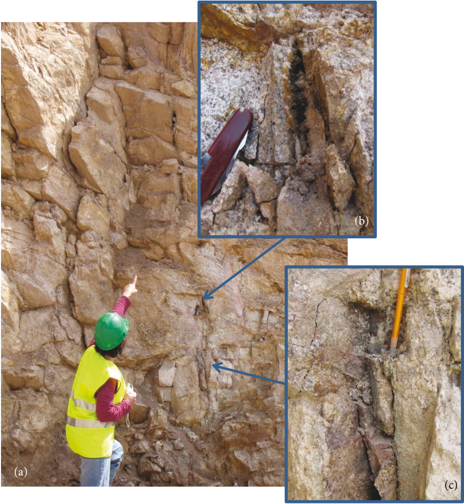
FIGURE 2: Example of fracture in granite (a) with quartz filling (b) and alteration halo (c) (Ottenhöffen quarry, Germany).
