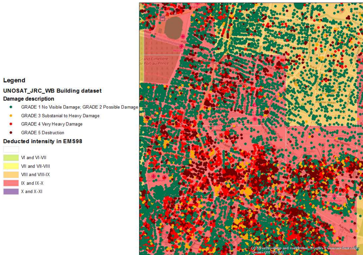
220 221 Figure 2: Close-up image of one district of Port-au-Prince. The back color represents the deduced 222 intensity. The dots represent the damaged buildings from the UWJ dataset.
