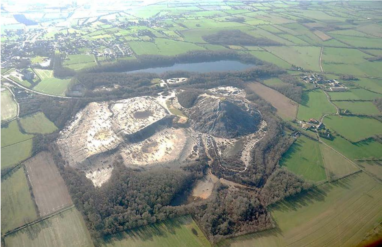
Figure 1 Aerial view of the site (tailings (left) and waste rocks (right) deposits, water-filled open pit)
