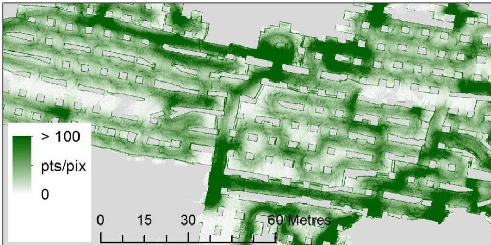
FIG. 7. Detailed view of point density (number of echoes per  $10\text{ cm} \times 10\text{ cm}$  cell) in a quarry extract. Density of 1 point/cm (score of 100 points/ $100\text{ cm}^2$ ) is mid-green. Darker greens show greater density. Such a view also highlights the path followed by the operator and demonstrate where geometric knowledge is best constrained.
