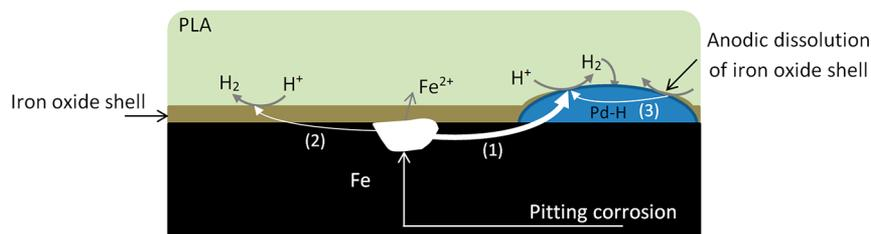
**Figure 1.** Schematic representation of the different corrosion currents which flow within nPd/ $\mu$ ZVI. (1) Main current which flows from Fe<sup>0</sup> to nPd. (2) Current which flows from Fe<sup>0</sup> to the oxide shell. (3) Current which flows from the oxide shell to nPd.
