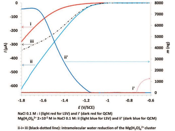
Fig. 1. Coupled LSV (left axis, curves i and ii) and QCM (right axis, curves i' and ii') measurements. Curve iii was obtained by subtracting curve ii from curve i.
