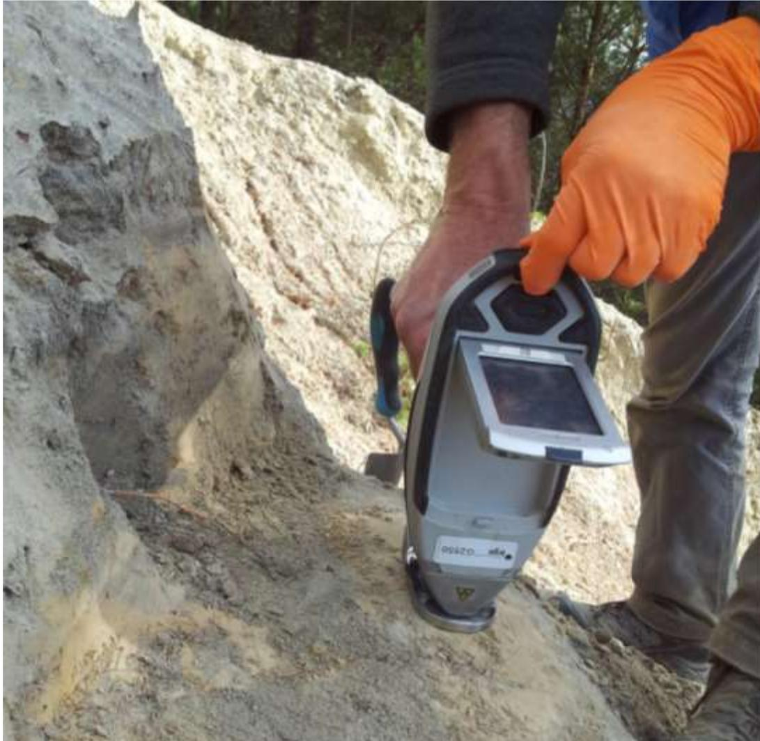
**Figure 4: On-site analysis of residues using pXRF**
