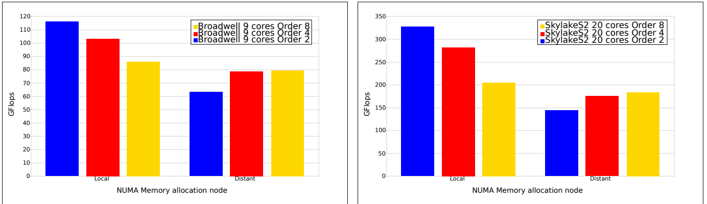
Figure 8: Comparison of local or remote memory access strategies with the indirect data access pattern on Broadwell and Skylake platforms.
