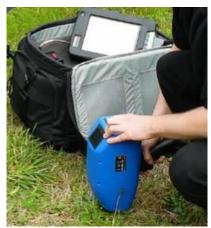
Figure 4: LIBS spectrometer (photo IVEA)
