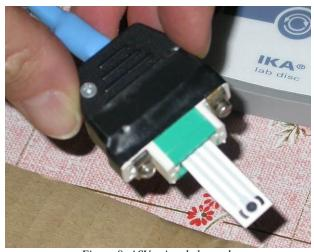
Figure 8: ASV printed electrode
