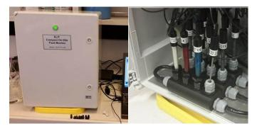
Figure 10: Fluid Management System consisting of a peristaltic pump and 12 ion selective electrodes (photo Nathan Reid, CSIRO)
