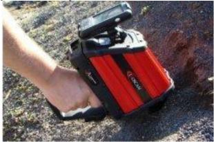
Figure 4: pFTIR spectrometer (photo Agilent)
