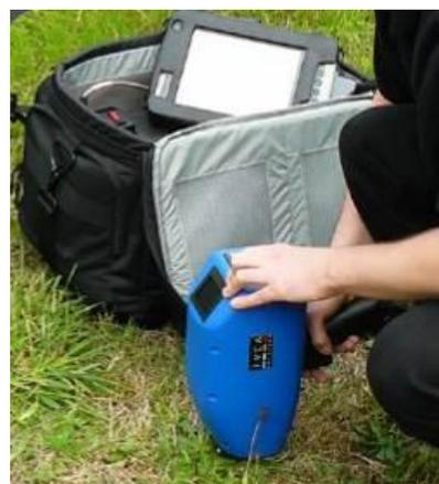
Figure 4: LIBS spectrometer (photo IVEA)
