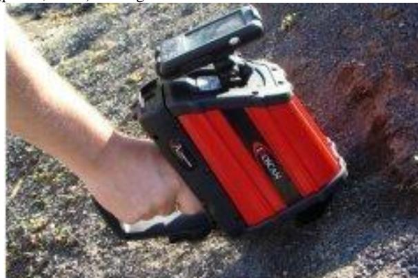
Figure 4: pFTIR spectrometer (photo Agilent)
