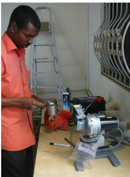
Figure 3: On-site battery operated sample milling device
