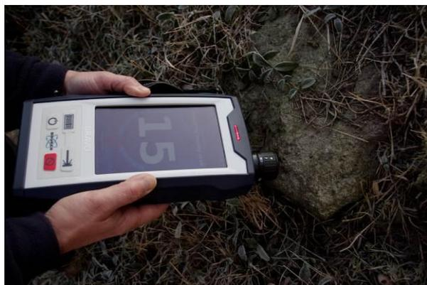
Figure 7:  $\mu$ Raman spectrometer (photo J. Jehlička)
