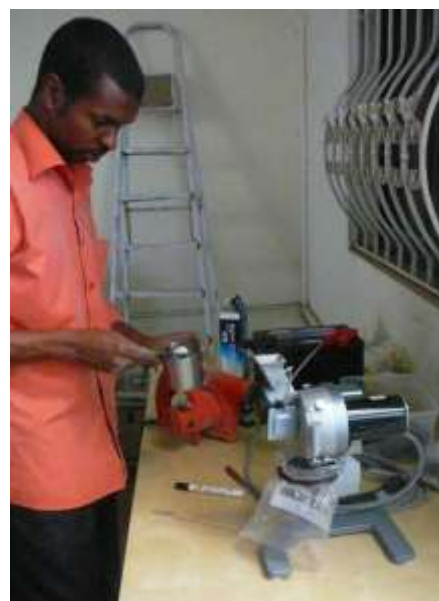
Figure 3: On-site battery operated sample milling device
