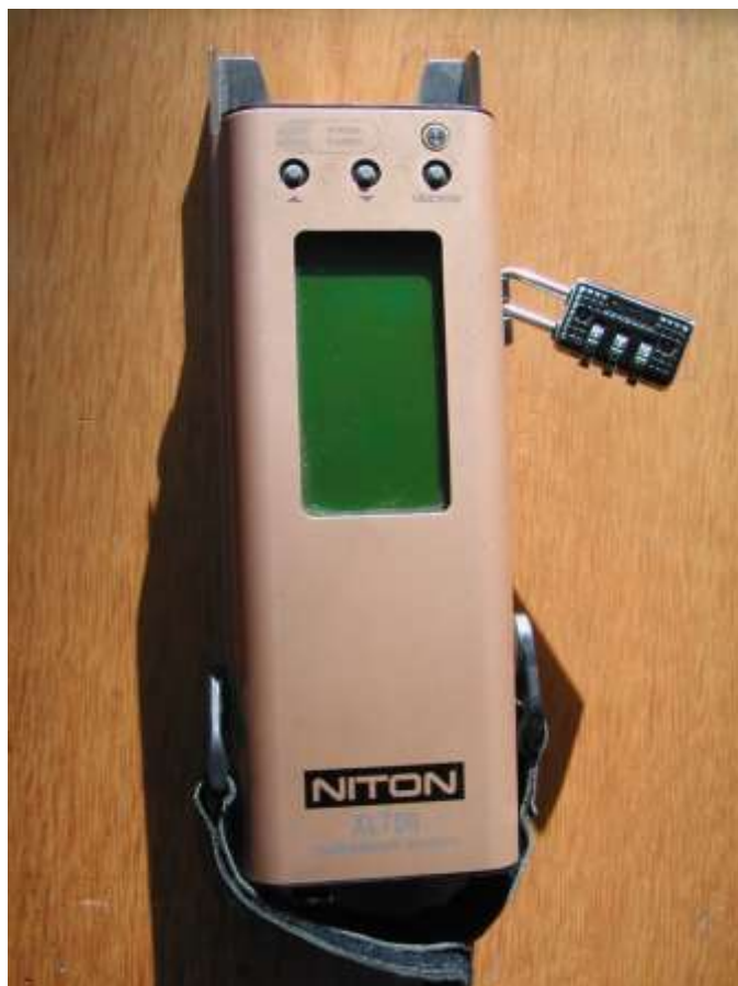
Fig. 1 An early radioactive source pXRF spectrometer
