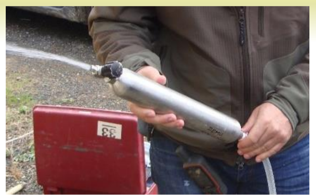
Figure 2 : sampling of waters for 14 C measurements with inox bottles
