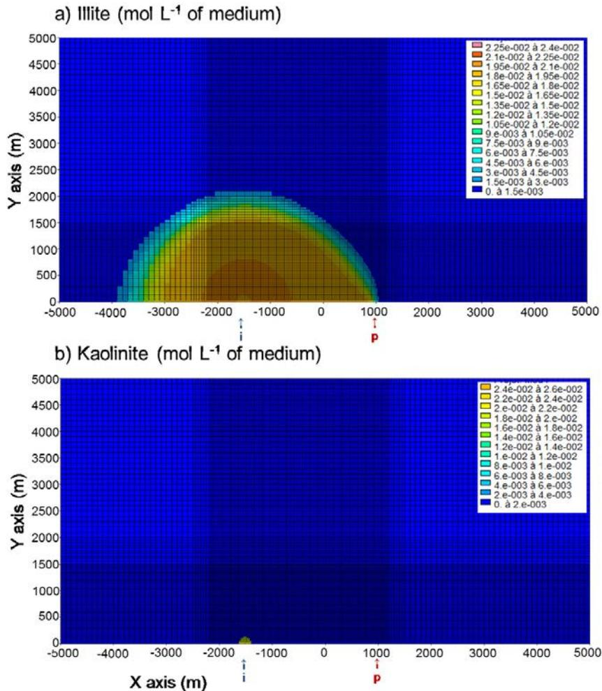
Fig. 7. Illite and kaolinite (mol L<sup>-1</sup> of medium) profiles in the clastic reservoir after 30 years of cooled and acidified water injection (MARTHE-PHREEQC calculation). i and p stand for the injection (-1,500 m) and production (1,000 m) wells, respectively.
