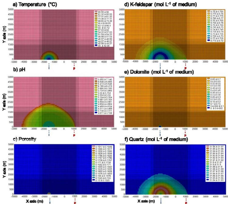
Fig. 6. Temperature (°C), pH, porosity, dolomite (mol L<sup>-1</sup> of medium), K-feldspar (mol L<sup>-1</sup> of medium) and quartz (mol L<sup>-1</sup> of medium) profiles in the clastic reservoir after 30 years of cooled and acidified water injection (MARTHE-PHREEQC calculation). i and p stand for the injection (-1,500 m) and production (1,000 m) wells, respectively.
