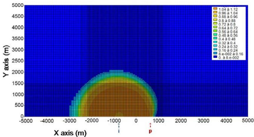
Fig. 5. C(4) concentration profile (mol L<sup>-1</sup>) in the carbonated reservoir after 30 years of cooled and acidified water injection (MARTHE-PHREEQC calculation). i and p stand for the injection (-750 m) and production (750 m) wells, respectively.
