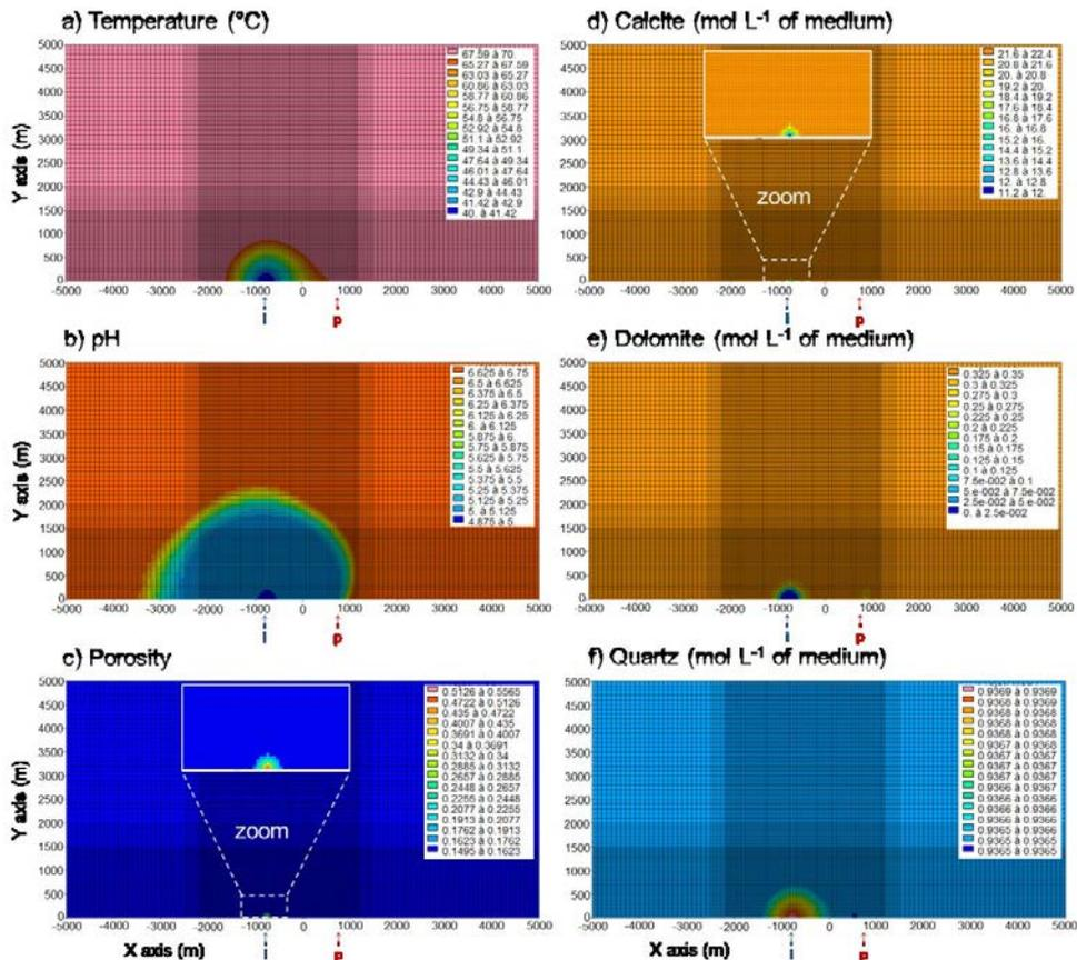
Fig. 4. Temperature (°C), pH, porosity, calcite (mol L<sup>-1</sup> of medium), dolomite (mol L<sup>-1</sup> of medium) and quartz (mol L<sup>-1</sup> of medium) profiles in the carbonated reservoir after 30 years of cooled and acidified water injection (MARTHE-PHREEQC calculation). i and p stand for the injection (-750 m) and production (750 m) wells, respectively.
