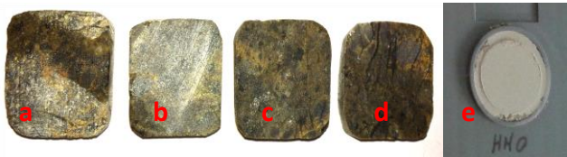
Figure 7: Peridotite samples – a: as-drilled; b: as-sawn; c: polished at 6 μm; d: polished at 0.25 μm; e: crushed to powder.
