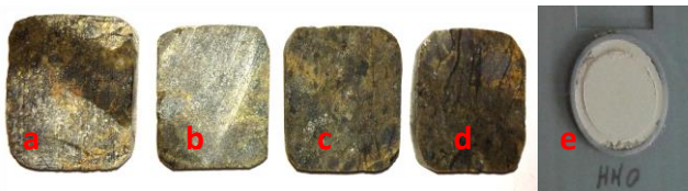
Figure 7: Peridotite samples – a: as-drilled; b: as-sawn; c: polished at 6 \mu\text{m} ; d: polished at 0.25 \mu\text{m} ; e: crushed to powder.
