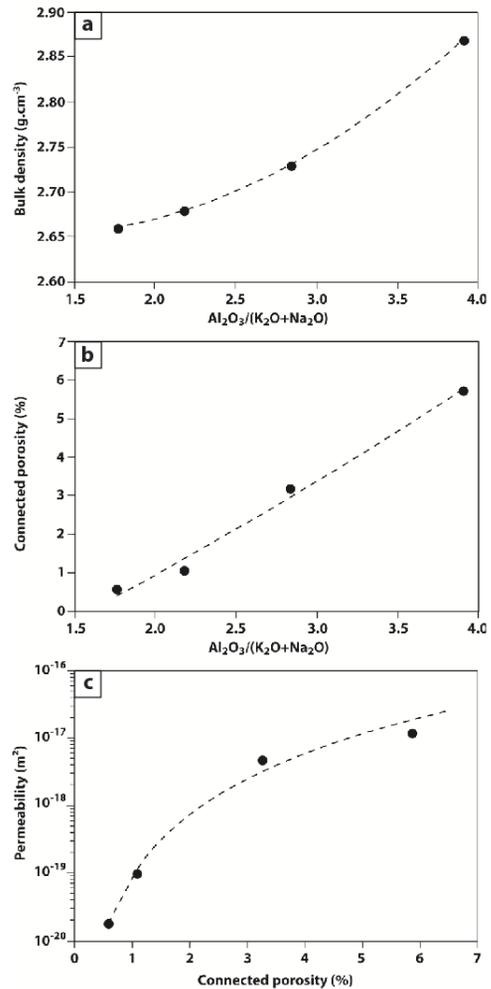
**Figure 3.** Evolution of **a** bulk density and **b** connected porosity in function of the alteration index  $Al_2O_3/(Na_2O+K_2O)$ . **c** Evolution of permeability in function of connected porosity.
