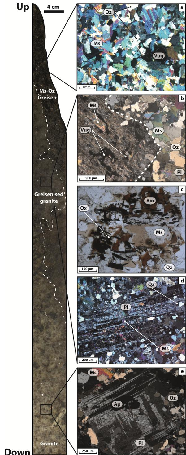
**Figure 2.** Zoned greisenisation of the Panasqueira granite in drill core section. **a** Section of the quartz-muscovite greisen endmember. **b** Section of K-feldspar replaced by muscovite. **c** Section of biotite bleached and partially transformed in muscovite. **d** Section of plagioclase partially altered and **e** section of fresh plagioclase in the unaltered granite.
