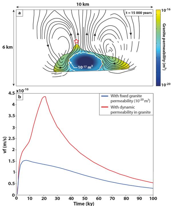
**Figure 4.** **a** Numerical solution (at 15 000 years) of fluid flow around granitic intrusion with dynamic permeability in the granite **b** fluid velocity above the apex (red star) between with fixed and dynamic permeability in the granite.
