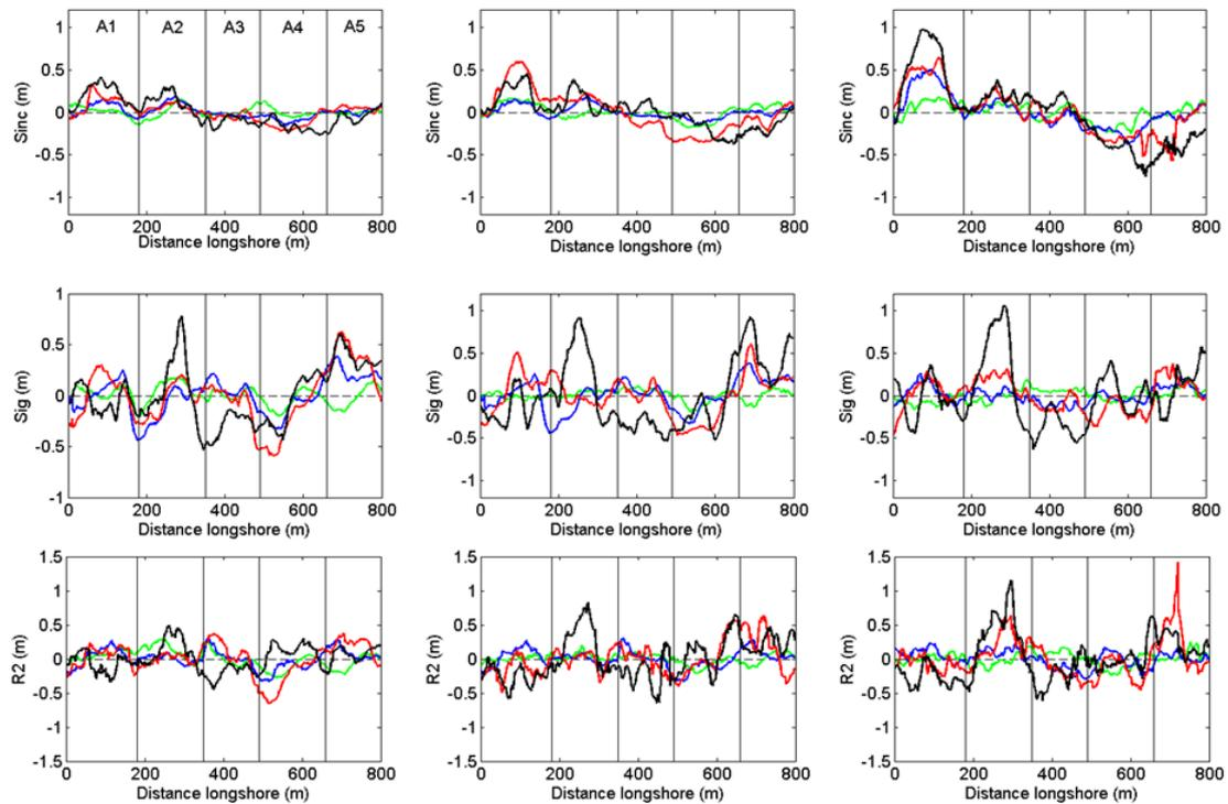
Figure 4 : Longshore local anomaly of  $S_{inc}$ ,  $S_{ig}$ ,  $R_{2\%}$  relative to respective longshore mean value. Left panel for mid-tide, center for mid-tide + 1m, right panel for high tide. Curve color: green for moderate conditions, blue for high conditions, red for storm conditions and black for extreme conditions.
