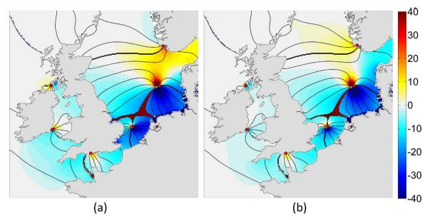
Fig. 7. M2 phase changes (in minutes) for SLR=2 m in comparison with the control scenario SLR=0 m, for the "no flood" (a) and "flood" (b) cases. Phases are plotted every hour. Thick lines indicate the 0 h phase, and the gray and red points indicate the amphidromic points for SLR=0 m and SLR=2 m, respectively.
