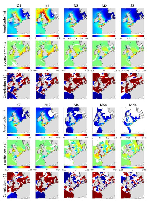
Fig. 3. Amplitudes of tidal components for the control scenario (SLR=0 m) (white: amplitudes smaller than 0.01); coefficients  $a_{CST_{amp}}$ , for areas of spatial similarity and proportionality (see the text for more explanation); maps of correlation coefficient r between  $\Delta\xi_{max}$  and  $\Delta CST_{amp}$  (red: r > 0; blue: r < 0; white: p-values  $\geq 0.05$ ).
