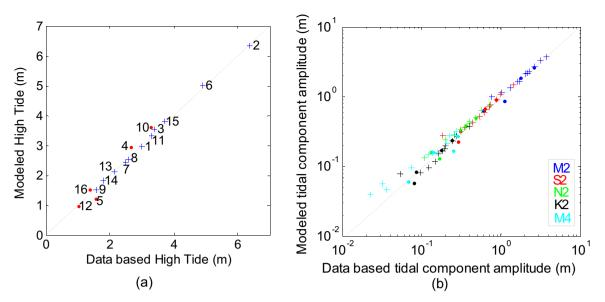
Fig. 2. (a) Modeled versus data-based highest annual tide (for the year 2009) for each site. The numbers refer to the tide gauge names (see Fig. 1a); (b) Modeled versus data-based tidal component amplitudes for 5 selected tidal components. + and • indicate sites with relative errors for the highest tide that are smaller or larger than 5%, respectively.
