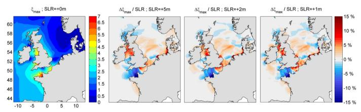
Fig. 5. Absolute values of maximum high tide level ( $\xi_{max}$ ) for the control scenario (SLR=0 m) and relative changes in the maximum water level ( $\Delta\xi_{max}$ /SLR).
