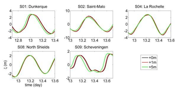
Fig. 4. Tidal curves from the S01, S02, S04, S07, S08, and S09 tide gauges (see Fig. 1a for locations) for a mean spring tide (equivalent to tidal forcing conditions occurring on 12–13 January 2009). These tide gauges are located in areas where tidal water level changes are proportional to SLR (see Section 3.1), in order to more easily illustrate the effects of SLR on the tides.
