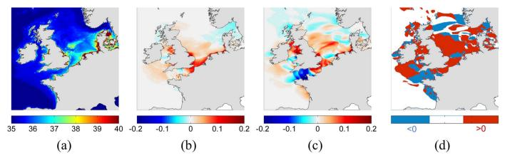
Fig. 9. (a) Strickler coefficient K(SLR=2) ( $m^{1/3} s^{-1}$ ); (b) changes in high tide level (m) for SLR=0 and K(SLR=2), i.e.,  $\Delta 1 = \xi_{max}(SLR=0, K(SLR=2)) - \xi_{max}(SLR=0, K_0)$ ; (c) changes in high tide level (m) for SLR=2 m and K<sup>\*\*</sup>K<sub>0</sub>, i.e.,  $\Delta 2 = \xi_{max}(SLR=2, K_0) - \xi_{max}(SLR=0, K_0)$ ; (d) sign( $\Delta 1$ )/sign( $\Delta 2$ ) (white:  $\Delta 1$  and  $\Delta 2$  smaller than 0.01 m).
