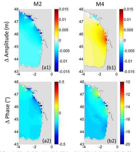
Fig. 13. Changes in tidal amplitude (1) and phase (2) for SLR=2 m, relative to SLR=0, for the M2 (a) and M4 (b) tidal components.
