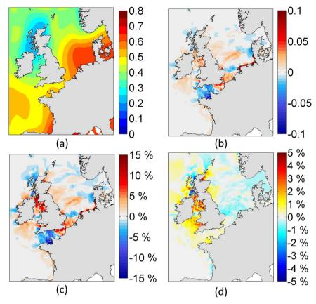
Fig. 14. (a) Non-uniform SLR (in meters); (b) absolute change  $\Delta \xi_{max}$  (in meters) for non-uniform SLR; (c) relative change  $\Delta 1 = (\Delta \xi_{max}/SLR)$  (in %) for non-uniform SLR; (d) relative difference  $(\Delta 1 - \Delta 2)/\Delta 2$  (in %) with  $\Delta 2 = (\Delta \xi_{max}/SLR)$  for SLR=0.5 m.
