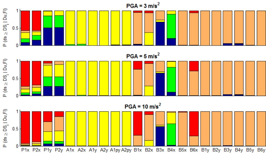
Fig. 7 – Distribution of component damage states given total functionality losses ( $F_i = 100\%$ ,  $D_u > 135$  days) and various seismic intensity. Damage states DS0 to DS4 are respectively represented by blue, green, yellow, orange and red bars.
