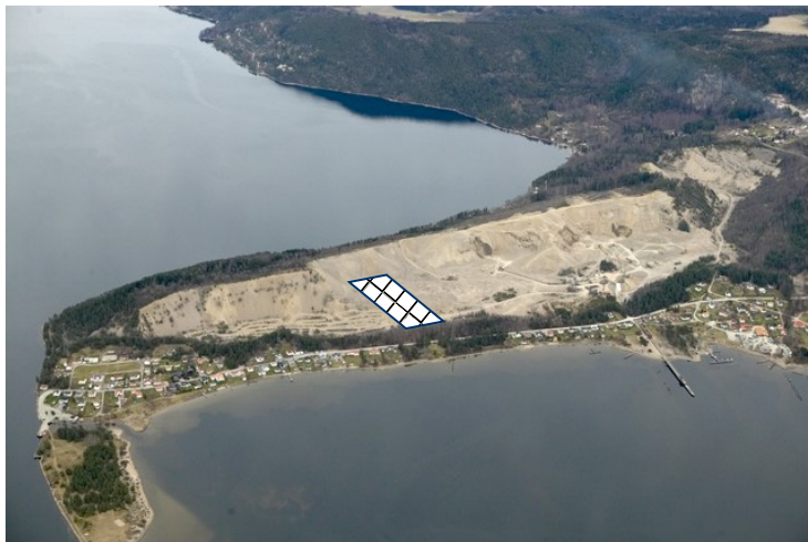
Figure 1. Aerial photo looking northwards on the Svelvik ridge at the outlet of the Drammensfjord. The ridge is formed by deglaciation deposits. The photo shows the sand excavation on the ridge. The location of the test site is indicated by the white rectangle (approximately 300 m by 150 m).
