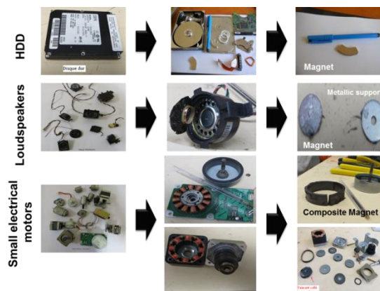
Figure 8: Recovery of magnet from different electronic components of WEEE by manual dismantling
