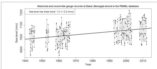
**Figure 9.** Monthly sea-level data available from the PSMSL repository for the two tide gauges in Dakar with associated linear trend (least-squares adjustment and formal uncertainties). Data recorded after 1992 originate from the most recent tide gauge.
