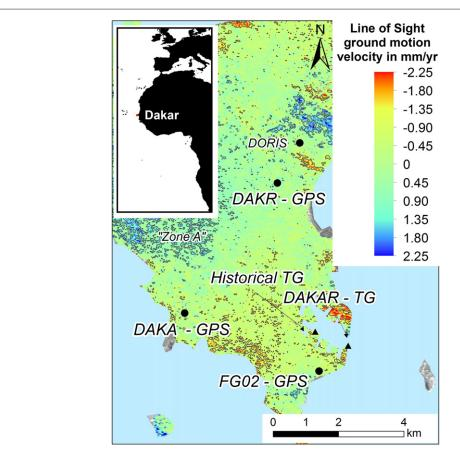
Figure 5. Line of Sight ground motion velocity in mm year $^{-1}$  for the whole 1993–2010 period (ERS1, ERS2 and Envisat). Negative values indicate subsidence. Gray contour lines are plotted for the following LoS ground motion velocity values:  $-3 \,$  mm year $^{-1}$ ;  $-1 \,$  mm year $^{-1}$ ;  $+1 \,$  mm year $^{-1}$ ;  $+3 \,$  mm year $^{-1}$ .
