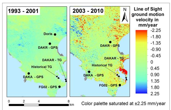
$\textbf{Figure 6.} \ Line of Sight ground motion velocity in mm year \\ ^{-1} for 1993-2001 \ (ERS 1-2 \ data, left) \ and \ 2003-2010 \ (Envisat \ data, right). \\ For figure readability, the color palette is saturated at its extreme values.$
