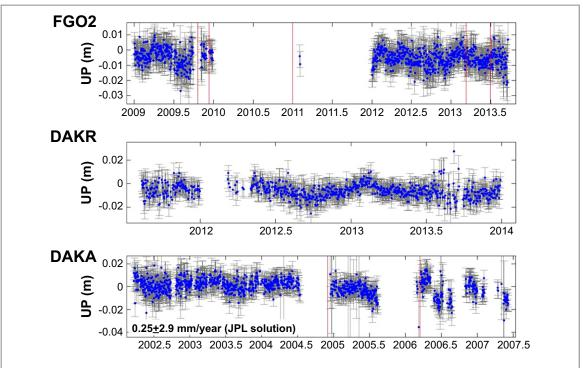
**Figure 4.** Records of the three GPS located in Dakar from the latest reprocessing of global GPS velocity fields of the University of La Rochelle (ULR-6). Red lines indicate discontinuities. In the case of the DAKA station, these discontinuities are probably related to changes of the instruments (see text).
