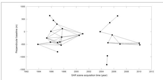
**Figure 3.** Baseline/time diagram for the ERS1, ERS2 and ENVISAT data. This diagram displays the selected SAR scenes (squares) and interferograms (segments) used to compute the following ground motion velocity maps. These scenes and interferograms meet the requirements in terms of baseline, time span, coherence and limited atmospheric effects. The ordinate axis origin is set to zero for the master scene of both Envisat and ERS stacks of interferograms (SAR scene acquired on 23rd October 2003).
