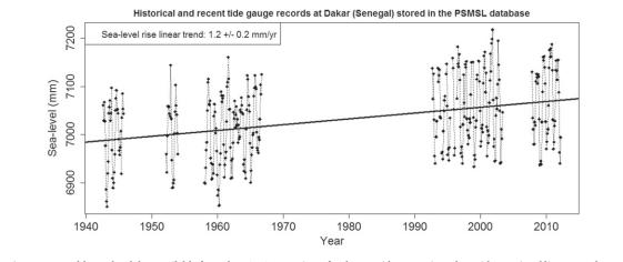
**Figure 9.** Monthly sea-level data available from the PSMSL repository for the two tide gauges in Dakar with associated linear trend (least-squares adjustment and formal uncertainties). Data recorded after 1992 originate from the most recent tide gauge.
