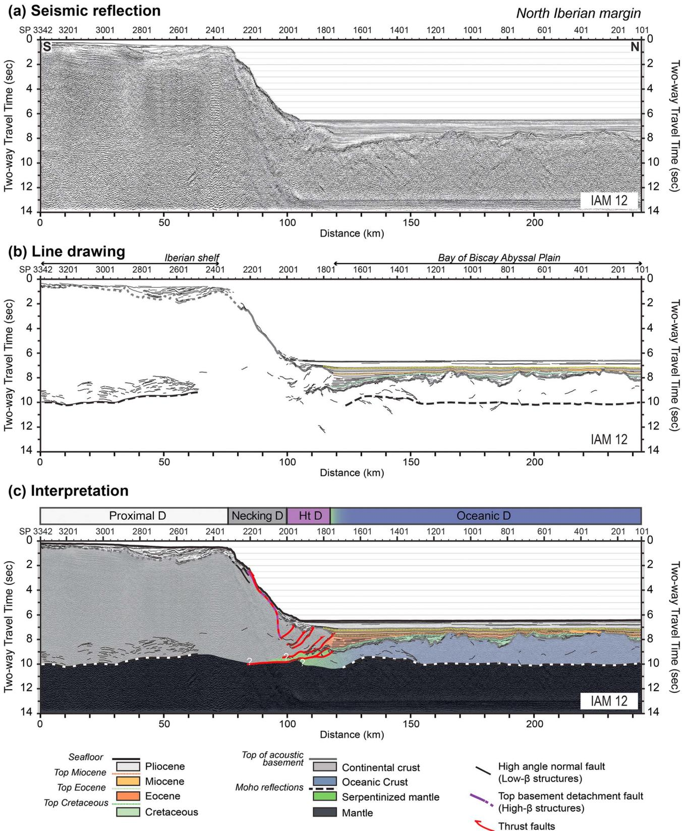
**Figure 9.** IAM 12 seismic section along the North Iberian margin. (a) Seismic reflection, (b) line drawing, and (c) interpretation proposed in this study. The location of the seismic lines is the same as Figure 7a.
