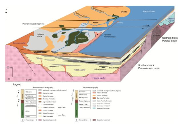
Figure 1: Schematic cross section of the geological study area (the vertical scheme has been modified from Maia et al., 2012).
