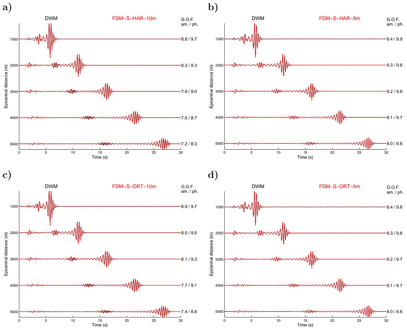
**Figure 20.** Vertical component of ground velocity along the northern surface profile for the 1D-smooth case computed with FDM-S using different grid spacings and definitions of the effective media: a) harmonic averaging, 10 m; b) harmonic averaging, 5 m; c) orthorhombic averaging, 10 m; d) orthorhombic averaging, 5 m.
