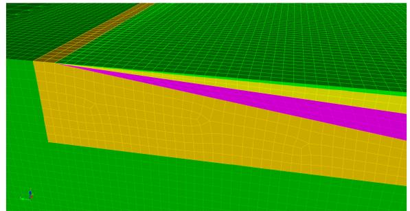
**Figure 21.** Spectral element mesh, designed following the F-strategy, used to compute a reference solution of the 2D-sharp case. The mesh consists of a 2-D section of unstructured quadrilaterals which is further “swept” along the direction transverse to the valley in order to define hexahedra. The mesh is further coarsened in the horizontal and vertical directions, from the orange “shoe-box” intermediate region to the outside green region.
