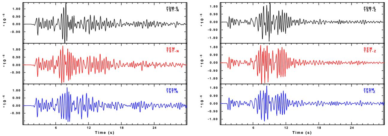
**Figure 3.** Same as Fig. 2 for the elastic model (neglecting intrinsic attenuation) with homogeneous layers. Note the good agreement on the first arrivals and the differences in phase and amplitude for later arrivals (between  $t = 6$  s and  $t = 12$  s).
