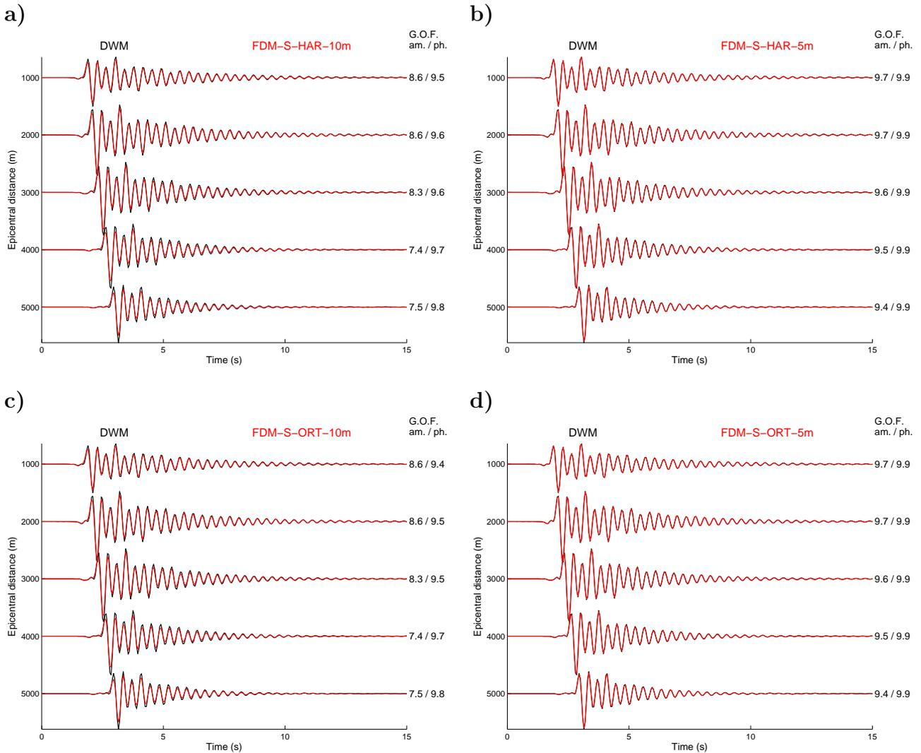
**Figure 15.** East-West component of ground velocity along the northern surface profile for the 1D-sharp case computed with FDM-S using different grid spacings and definitions of the effective media: a) harmonic averaging, 10 m; b) harmonic averaging, 5 m; c) orthorhombic averaging, 10 m; d) orthorhombic averaging, 5 m.
