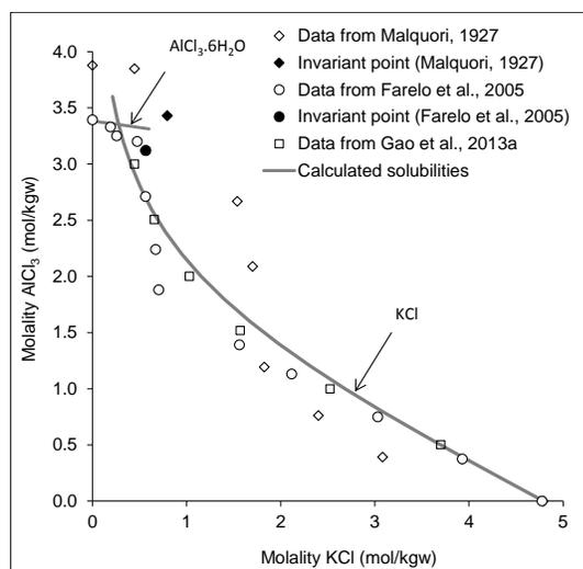
**Fig. 2:** Salt solubility diagrams in (KCl+AlCl<sub>3</sub>) solutions at 25°C
