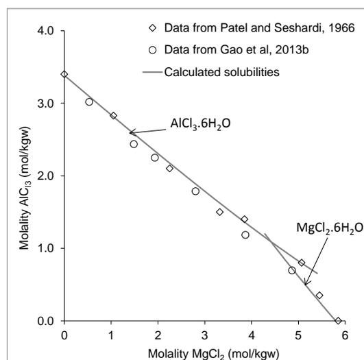
**Fig. 3:** Salt solubility diagrams in (MgCl<sub>2</sub>+AlCl<sub>3</sub>) solutions at 25°C
