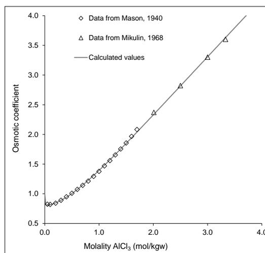
**Fig. 1:** Calculated (line) and experimental (symbols) water activity for the AlCl<sub>3(aq)</sub>-H<sub>2</sub>O binary system as a function of total molality of AlCl<sub>3</sub> at 25 °C. The maximum experimental ionic strength is about 20 eq/kg.
