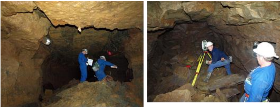
Figure 7: visit underground of an area at risk for sink holes (BRGM)
