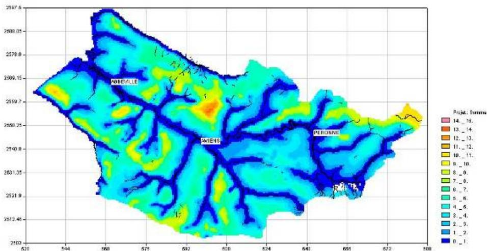
The model has shown that the contribution of compartments of the chalk aquifer to the Somme discharge increased proportionally upstream to downstream. While the groundwater contribution to stream flow during the summer months is nearly 100%, it was estimated to have accounted for around 80% during the 2001 flood.
