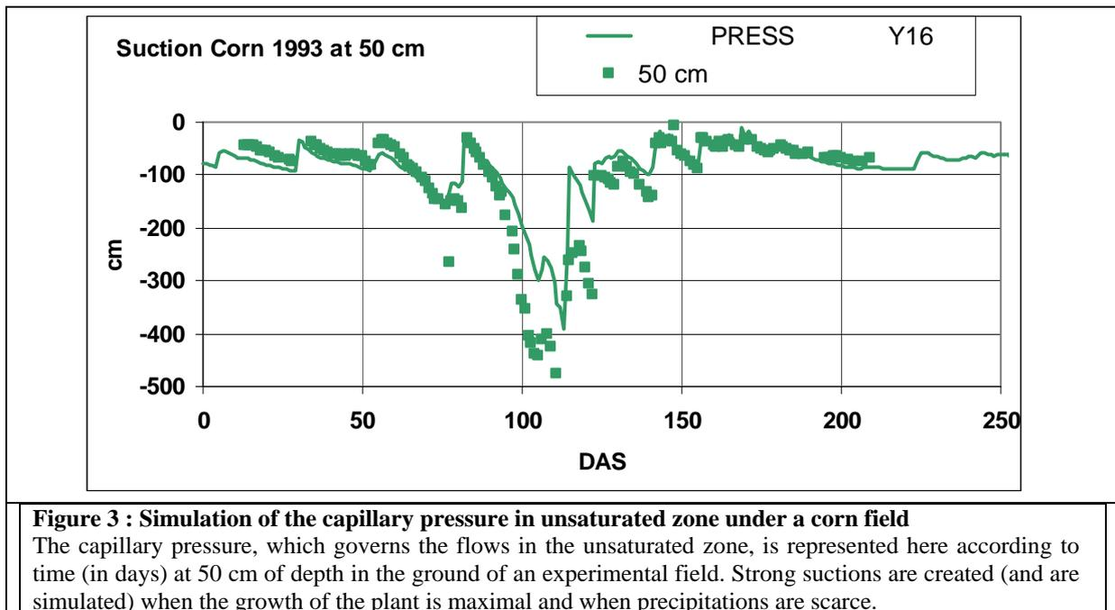
**Figure 3 : Simulation of the capillary pressure in unsaturated zone under a corn field**
