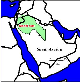
The Saq aquifer is a huge sandstone reservoir, over 375 000 sq Km (2/3 of France total area), in the North of Saudi Arabia. This area counts about 16 000 wells out of which only 600 are used for drinking water supply, the rest being used for irrigation in the desert.
