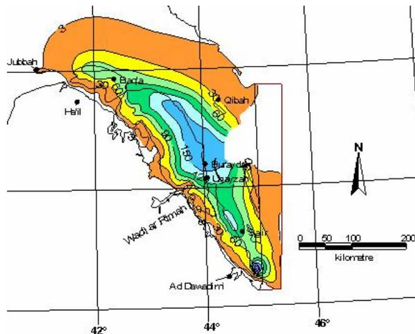
The model spots the areas affected by abstraction between 1960 and 2005, where huge drawdown take place. As aquifer recharge is very weak (0 to 5 mm/a), any significant groundwater abstraction is clearly a mining operation.
