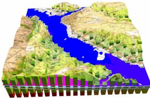
The Somme river valley (France): 3D representation of the 2001 flood in the south of Abbeville. The cells are represented by parallelepipeds. The geological map is draped over. Fine overflowing cells are coloured in blue to represent flooded areas.
