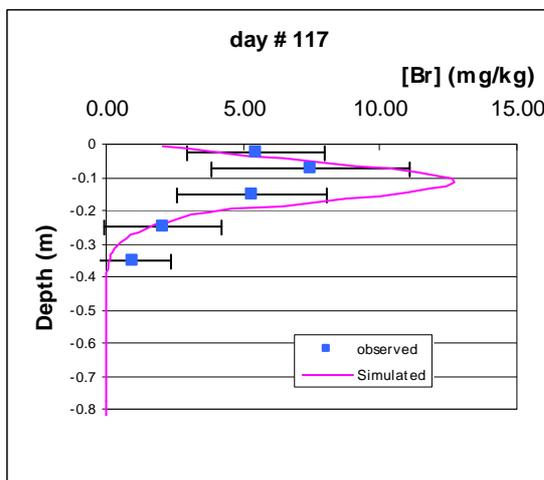
Bromide can be considered as perfect tracer and proper simulation of flow is the condition of success. Although extremely simplified, the 1D modelling globally respects the concentrations and delay of Bromide transfer, 7 days after application.
