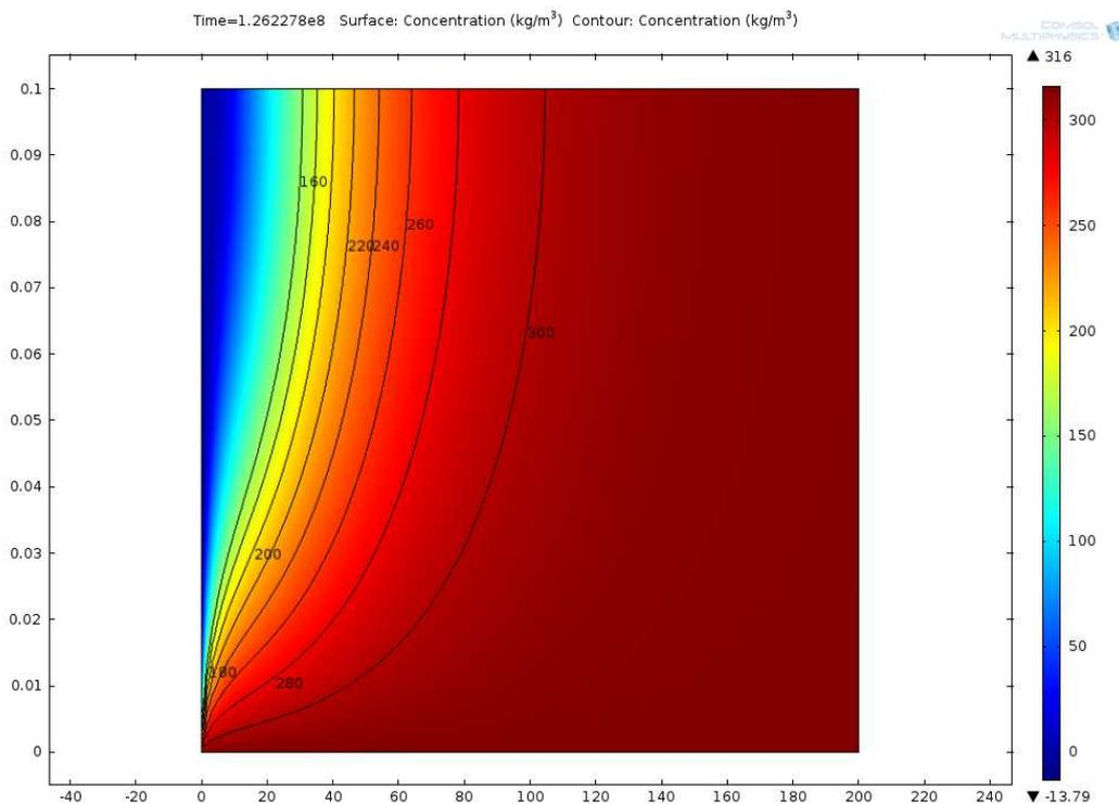
**Figure 2** Calculated concentration field (hyd. cond. = 10<sup>-3</sup> m/s, hyd. gradient = 0.4 %).
