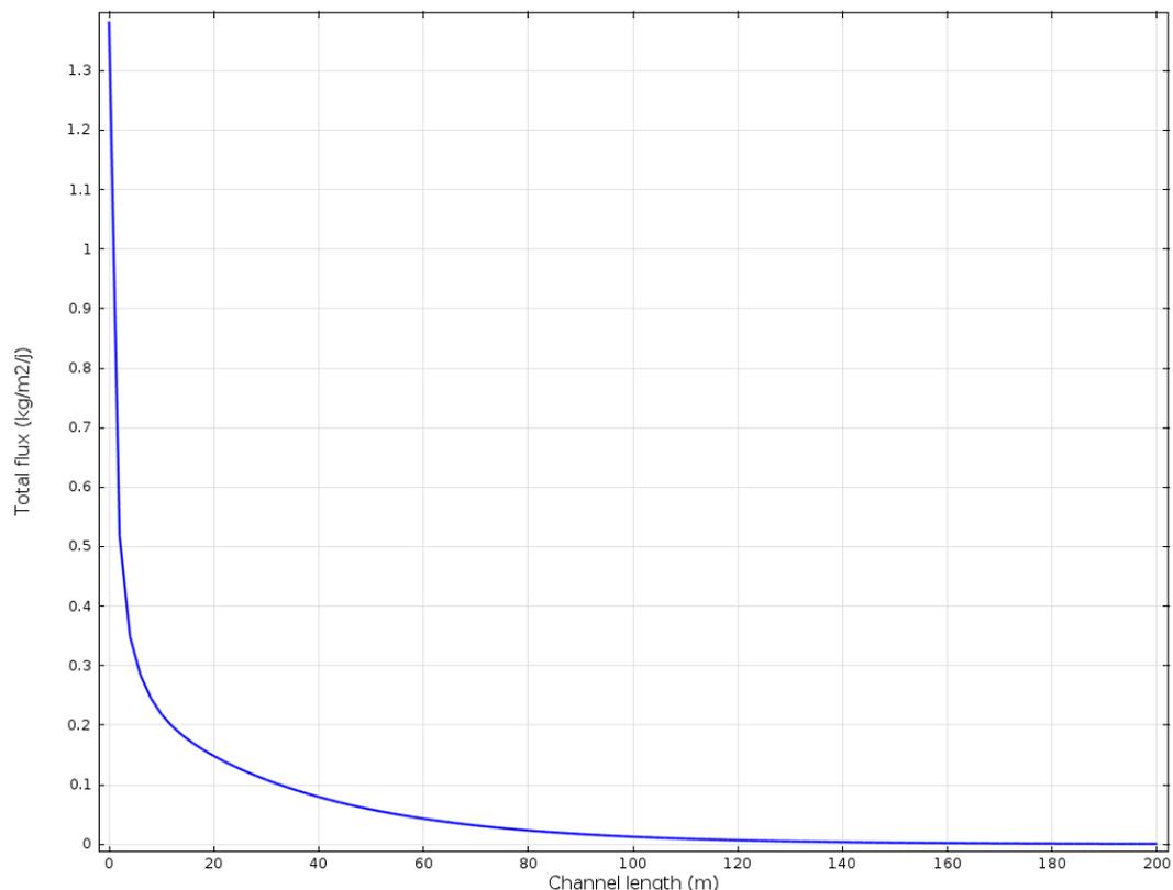
**Figure 3** Calculated dissolution flux at lower boundary (hyd. cond. =  $10^{-3}$  m/s, hyd. gradient = 0.4 %).
