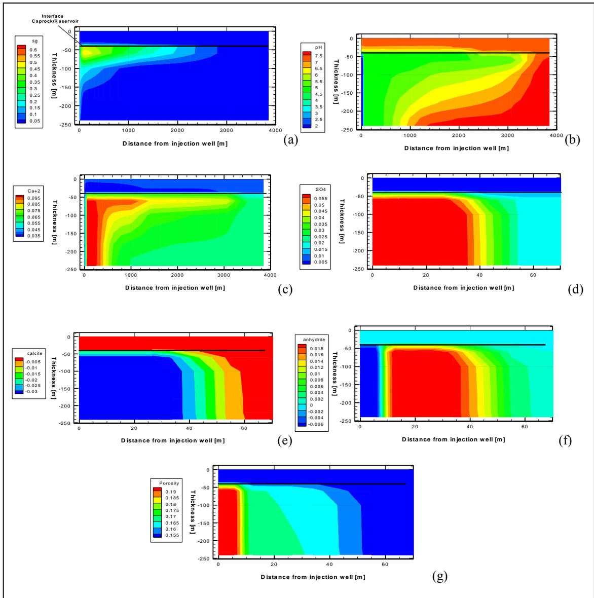
Figure 3. State of the reservoir and caprock after a 30-year injection period. a) Gas saturation ( $S_g$ ), b) pH pattern, c) Calcium concentration ( $\text{mol/kg}_{\text{H}_2\text{O}}$ ) with x-axis up to 4000 m, d) Sulfate concentration ( $\text{mol/kg}_{\text{H}_2\text{O}}$ ), e) Volumic fraction of calcite, f) Volumic fraction of anhydrite, g) Porosity with x-axis up to 70 m from injection well
