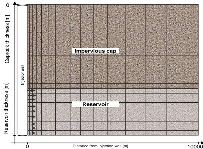
Figure 2. The geometrical 2-D radial model (vertical cross-section)
