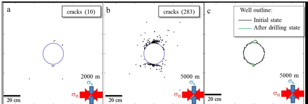
**Figure 4: Cracks in the hydrothermally altered granite following the well drilling-induced discharge at 2,000 m deep (a) and at 5,000 m deep (b). c: Change in the well outline at 5,000 m resulting from the cracks coalescence.**
