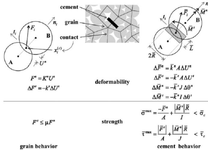
**Figure 1: Force–displacement behavior of the particles (grain behavior) and of the parallel bonds (cement behavior; Potyondy and Cundall, 2004)**
