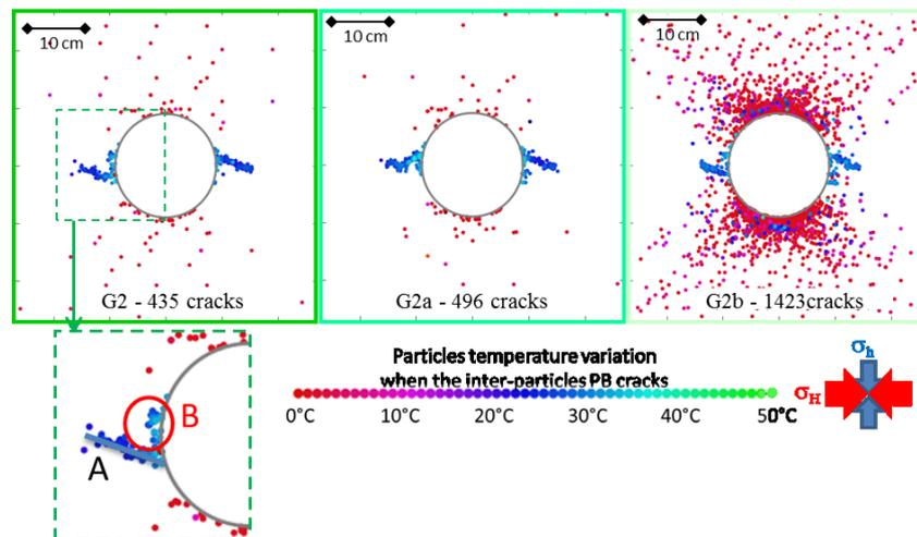
**Figure 8: Simulated cracks in the sandstones after 6 hours of thermal loading over-imposed to cracks due to drilling process. A and B on zoomed view: A is the major tensile fracture and B localizes secondary aborted tensile fractures**
