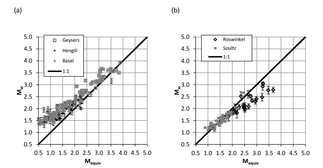
Figure 9: Comparison of common  $M_{equiv}$  versus inverted  $M_w$  for all datasets in the study. (a) Geysers, Hengill and Basel events. (b) Roswinkel and Soultz events.
