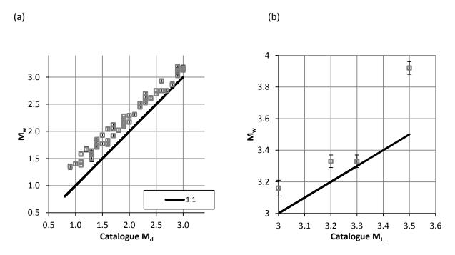
Figure 3: Comparison of moment magnitude  $(M_w)$  versus catalogue (a) duration magnitude  $(M_d)$  and (b) local magnitude  $(M_L)$  for the Geysers dataset.
