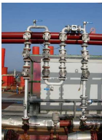
Figure 12: Corrosion and coating study with the High Temperature Skid installed on the Soultz plant (picture GEIE).
