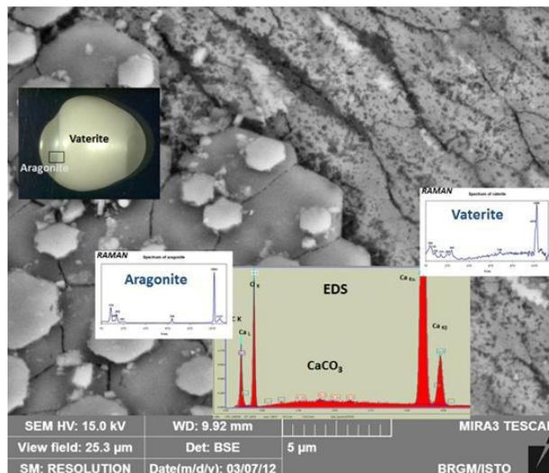
***SEM picture of pearl surface at the interface of the defect (inset is the pearl, squared is the zone observed); superposed are the EDS spectrum of CaCO<sub>3</sub> on both sides and Raman spectra showing the different polymorphs.***
