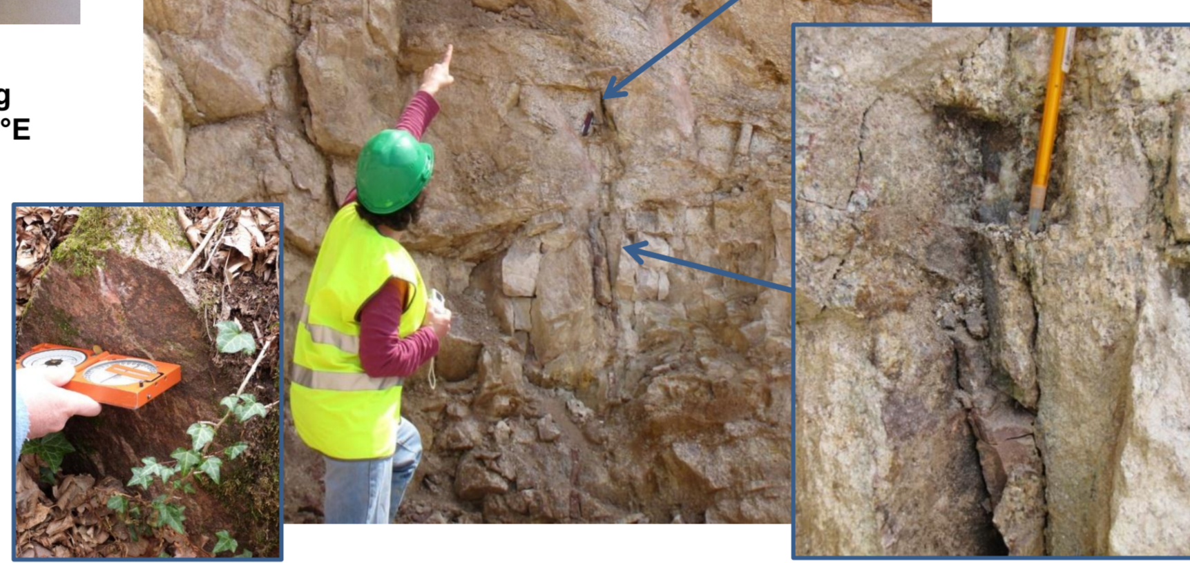
Fracture in granite with quartz filling and alteration halo (Ottenhöfen quarry, Germany)
