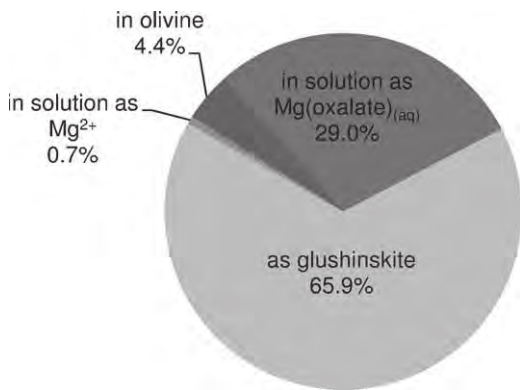
Fig. 14. Speciation of magnesium from first simulation assuming instantaneous precipitation of amorphous silica ( 3 \text{ g l}^{-1} slurry with 0.1 \text{ M} oxalate salt, under 120^\circ \text{C} and 20 \text{ bar} of \text{CO}_2 ).
