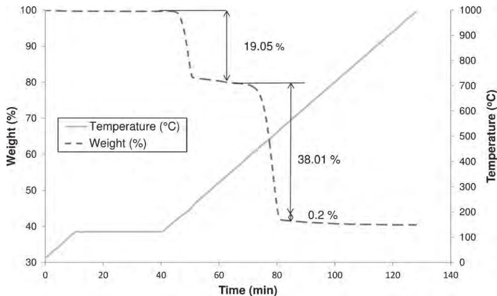
**Fig. 5.** Thermogravimetric analysis of final solid product consisting mainly of magnesium oxalate dihydrate. Two characteristic mass losses are observed: between 120 °C and 300 °C water is released; between 300 °C and 600 °C dehydrated oxalate decomposes into CO<sub>2</sub> and CO.
