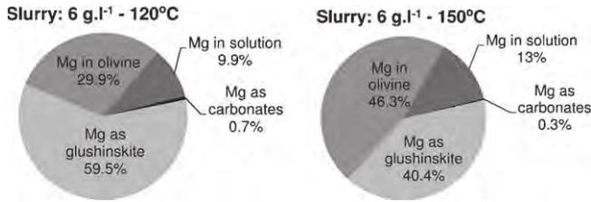
**Fig. 10.** Extraction yield and speciation of magnesium after 24 h with 6 g l<sup>-1</sup> slurry at 120 °C and 150 °C (0.1 M oxalate salt, 20 bar of CO<sub>2</sub>).
