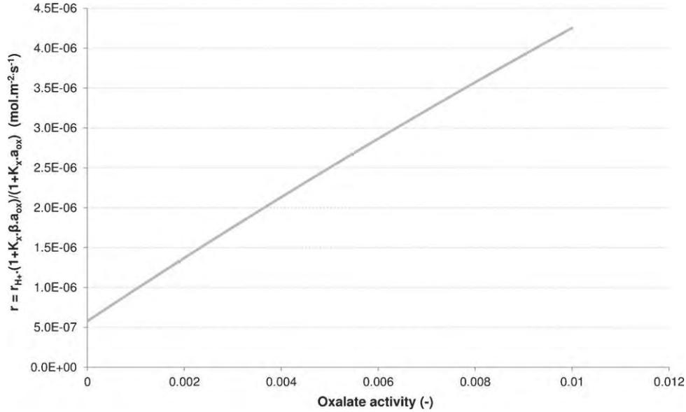
**Fig. 1.** Oxalate-promoted dissolution rate at 120 °C according to the rate law given by Prigiobbe and Mazzotti (2011): evolution as a function of oxalate activity in solution (with constant proton activity set to  $8.7 \times 10^{-6}$ , rate without additive being  $r_{H^+} = 5.8 \times 10^{-7} \text{ mol m}^{-2} \text{ s}^{-1}$ ).
