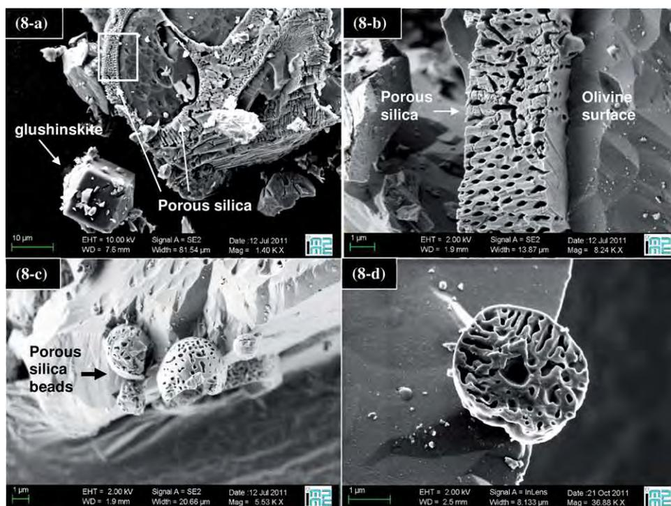
**Fig. 8.** FEG-SEM images of solid particles after 1 h of reaction ( $3 \text{ g l}^{-1}$  slurry with 0.1 M oxalate salt, under  $120^\circ \text{C}$  and 20 bar of  $\text{CO}_2$ ). (a) An olivine particle partially covered by a porous silica layer; glushinskite crystals are observed. (b) The microstructure of the highly porous precipitated silica layer. (c and d) Micrometric porous silica beads on the olivine surface.
