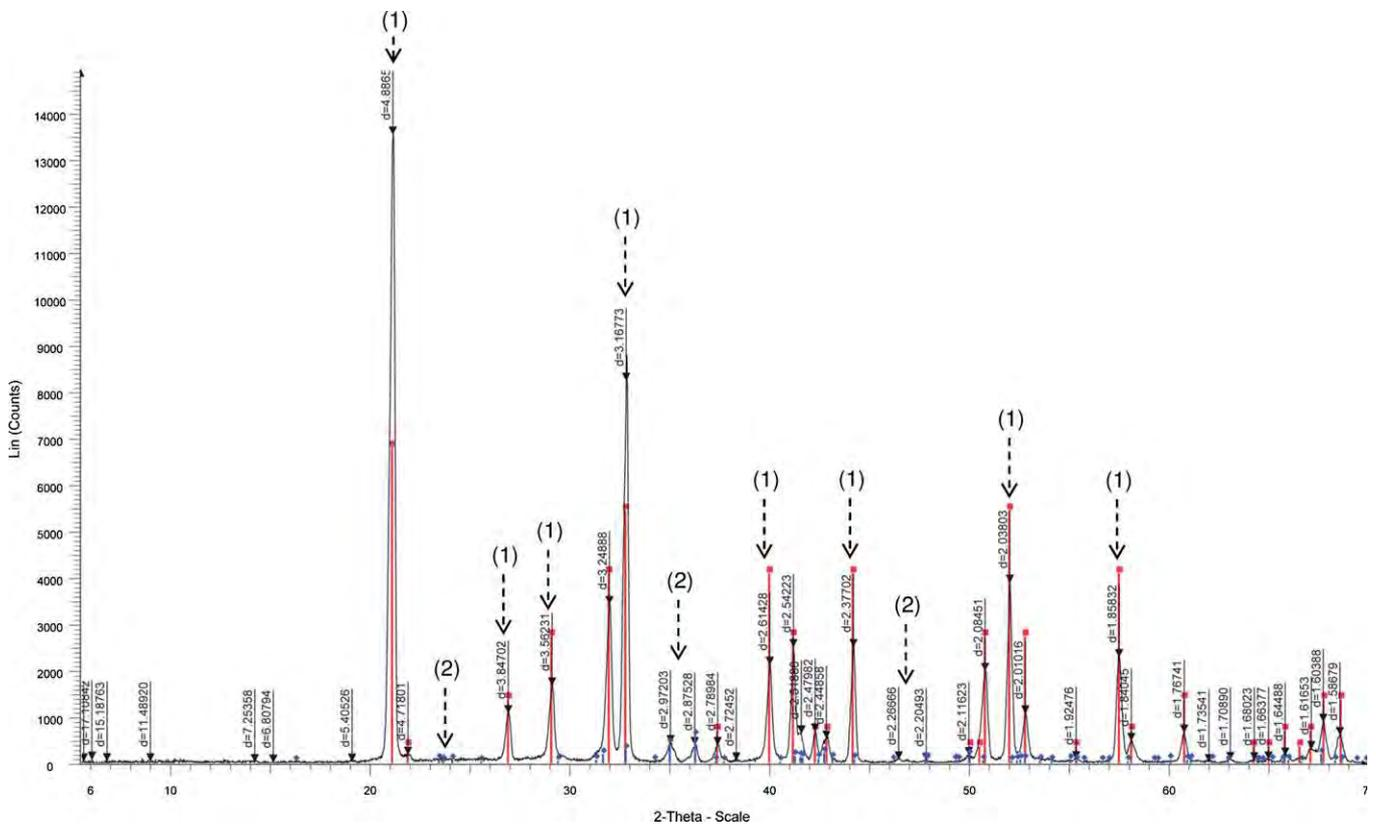
**Fig. 4.** X-ray diffraction pattern of final solid product under dilute slurry conditions ( $3 \text{ g l}^{-1}$  of olivine with  $0.1 \text{ M}$  disodium oxalate,  $120^\circ \text{C}$  and  $20 \text{ bar}$  of  $\text{CO}_2$ ). (1)  $\alpha\text{-Mg}_2\text{O}_4 \cdot 2\text{H}_2\text{O}$  (23-0394) or synthetic glushinskite, (2) clinoenstatite (35-0610) (traces) from initial material.
