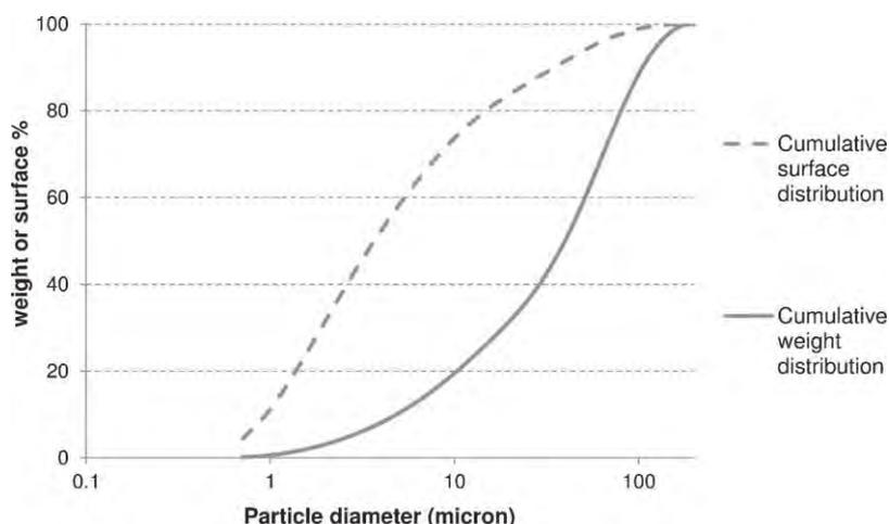
Fig. 2. Cumulative particle size distribution by mass and by surface for ground olivine sieved under  $100\ \mu\text{m}$ .
