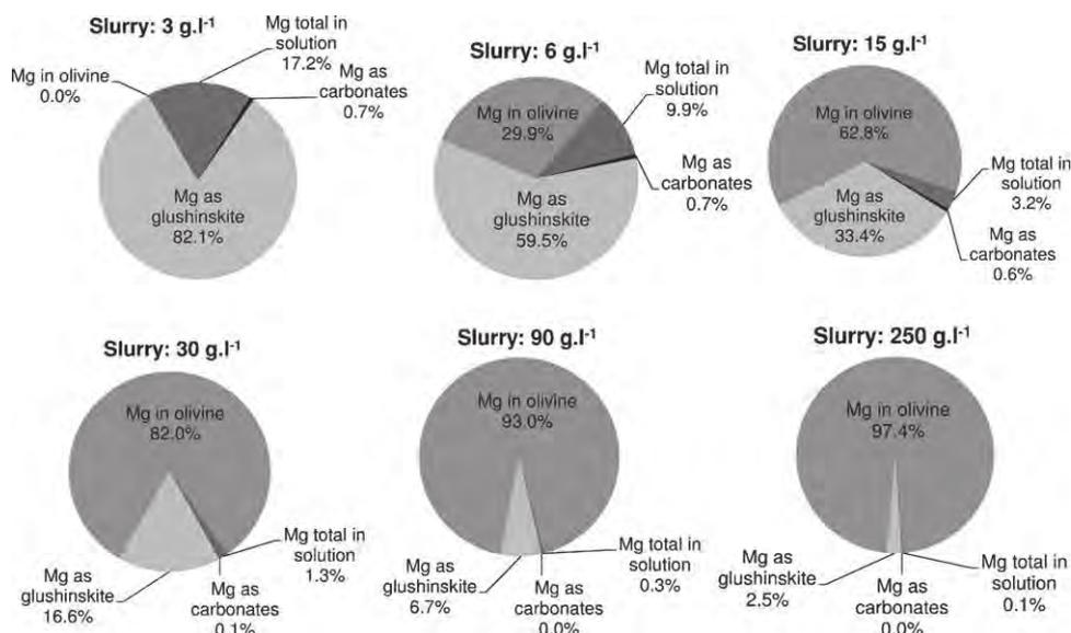
**Fig. 6.** Magnesium speciation as a function of slurry concentration after 24 h of batch reaction (0.1 M disodium oxalate, 120 °C, 20 bar of CO<sub>2</sub>, initial particle size below 100 μm).
