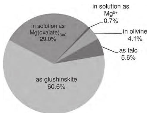
**Fig. 16.** Predicted speciation of magnesium after 24 h of reaction when accounting for precipitation kinetics of amorphous silica and talc ( $3 \text{ g l}^{-1}$  slurry with  $0.1 \text{ M}$  oxalate salt, under  $120^\circ \text{C}$  and  $20 \text{ bar}$  of  $\text{CO}_2$ ).
