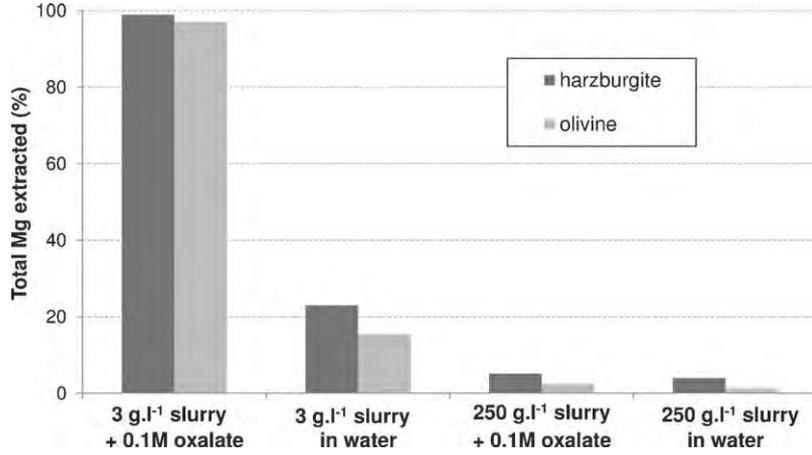
**Fig. 12.** Comparison of magnesium extraction yields in water and with 0.1 M oxalate, for olivine and harzburgite (3 g l<sup>-1</sup> and 250 g l<sup>-1</sup> slurries under 120 °C and 20 bar of CO<sub>2</sub>).
