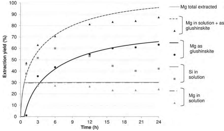
**Fig. 13.** Comparison between experimental data and shrinking particle simulation results assuming instantaneous precipitation of amorphous silica ( $3 \text{ g l}^{-1}$  slurry with  $0.1 \text{ M}$  oxalate salt, under  $120^\circ \text{C}$  and  $20 \text{ bar}$  of  $\text{CO}_2$ ).
