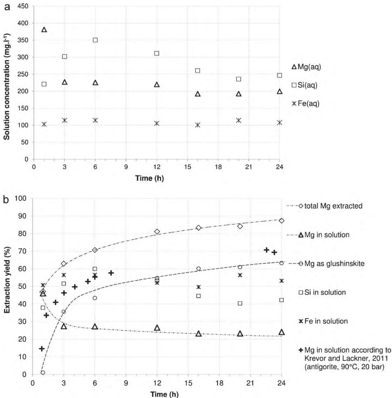
**Fig. 7.** Evolution of aqueous species concentration (Mg, Fe and Si) (a) and of extraction yields with Mg speciation (b) ( $3 \text{ g l}^{-1}$  olivine slurry with  $0.1 \text{ M}$  oxalate salt, under  $120^\circ\text{C}$  and  $20 \text{ bar}$  of  $\text{CO}_2$ ).
