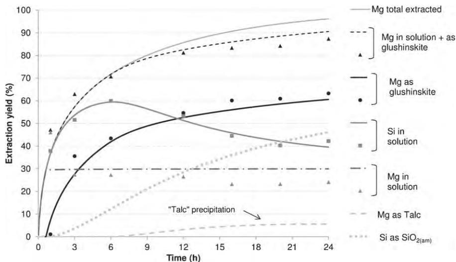
**Fig. 15.** Comparison between experimental data and shrinking particle simulation results when accounting for precipitation kinetics of amorphous silica and talc ( $3 \text{ g l}^{-1}$  slurry with  $0.1 \text{ M}$  oxalate salt, under  $120^\circ \text{C}$  and  $20 \text{ bar}$  of  $\text{CO}_2$ ).
