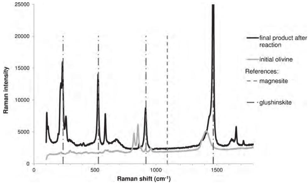
**Fig. 3.** Raman spectra showing glushinskite precipitation under dilute slurry conditions ( $3 \text{ g l}^{-1}$  of olivine with  $0.1 \text{ M}$  disodium oxalate, under  $120^\circ \text{C}$  and  $20 \text{ bar}$  of  $\text{CO}_2$ ).
