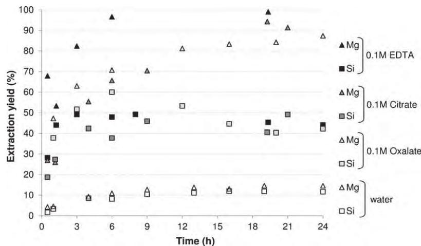
**Fig. 11.** Total amount of magnesium and silicium extracted for various aqueous solutions: without additive, with 0.1 M of respectively, oxalate, citrate or EDTA salt (3 g l<sup>-1</sup> slurry with particle size <100 μm, under 120 °C and 20 bar of CO<sub>2</sub>).
