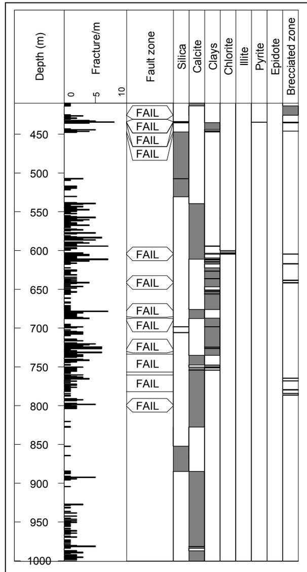
Figure 7. Fracture density, major fault location, and vertical distribution of the hydrothermal fillings sealed fractures in the Californie well.
