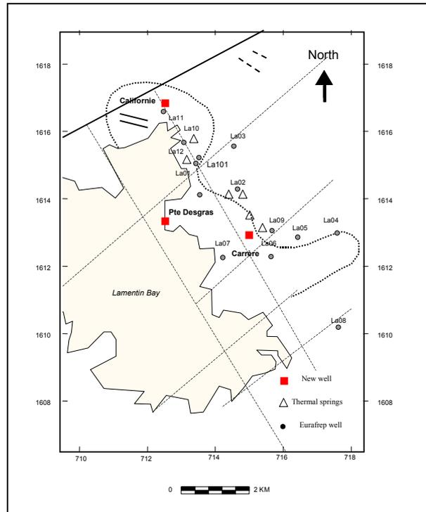
Figure 2. Map showing the locations of the thermal springs, the old and the recent geothermal wells, the fault system and the envelope of the geochemical anomalies in As, Hg, CO<sub>2</sub>, Helium (dotted line).
