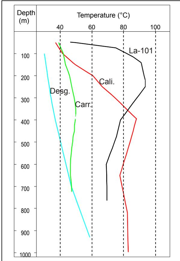
Figure 3. Representative temperature profile measured in the 4 deep wells drilled in the Lamentin area.
